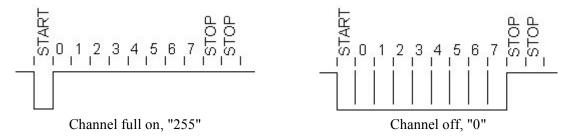
Each channel is separated by a logic "high" or "mark" partition between the 8-bit data byte.
