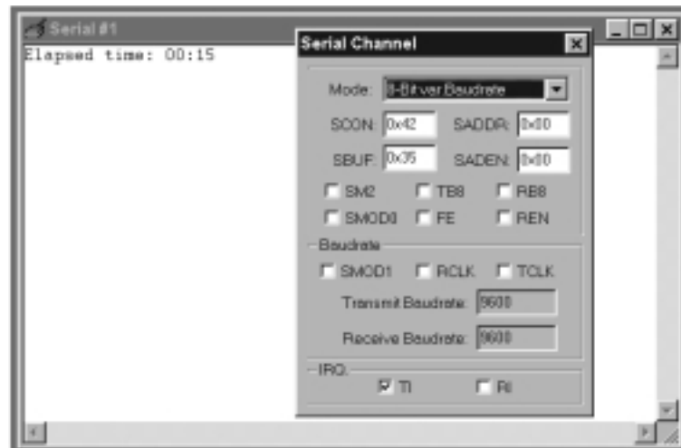
FIGURE 9.3 Output from a simple 'output only' PC-link library, running under the Keil hardware simulator. See text for details
