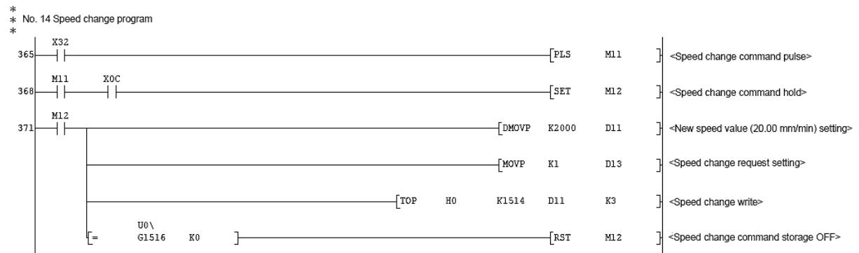
(g) Speed change using overwrite function (QD75 additional function)
