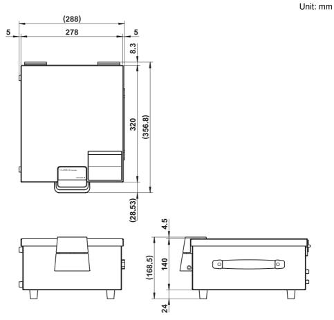
Unless otherwise specified, tolerance is  $\pm 3\%$  (however, tolerance is  $\pm 0.3$  mm when below 10 mm).
