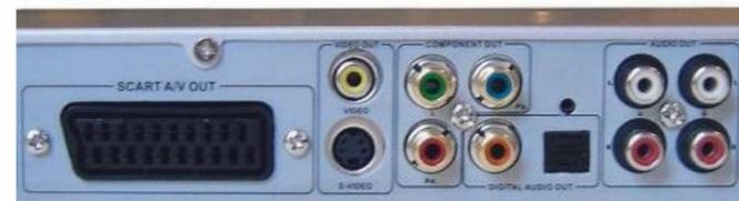
**Europe:** Using the SCART cable included in the package, insert the SCART output of the ShowCenter Player into the SCART input on your TV. If possible, the SCART connection of your TV should support RGB signals since this delivers the best picture quality. You should switch to SCART-RGB later via the ShowCenter Player Settings menu.
