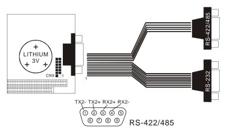
Note : TX2+,TX2- and RX2+,RX2- are for transmitting and receiving, respectively, in the RS-422 connection. While in RS-485 connection, TX2+,RX2+ and TX2-,RX2- must be twisted each. Anyhow, you can only choose to use **RS-232** or **RS-422/485**.
