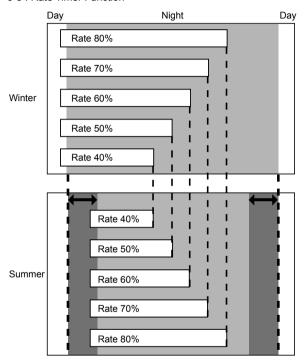
**SolarAmp mini** rate timer is different from a traditional night-light timer. The lighting time of load is set by a rate (%) of night time. Even if the night time is changed seasonally, the lighting-off time will be apporoximately at the same time. There is no need to reset the timer setting as seasons change.
