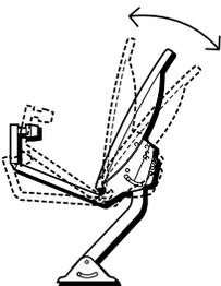
*Elevation is the up/down angle that the satellite dish antenna is pointed.*
