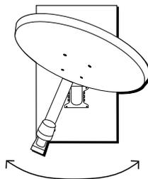
*Azimuth is the side-to-side direction that the satellite dish antenna is pointed.*
