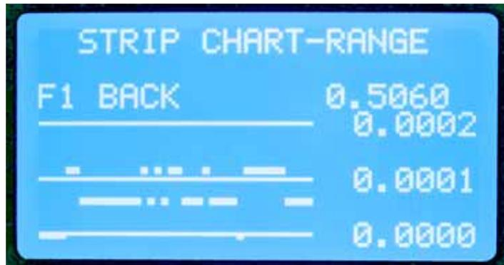
The *range*, the difference between the longest and the shortest spring in the sample, is plotted on the R chart.
