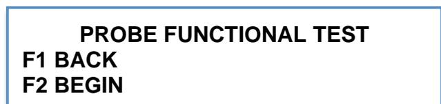
If a failure is found, you will be prompted to disconnect the probe from the gage. Contact LSI regarding repairs.
