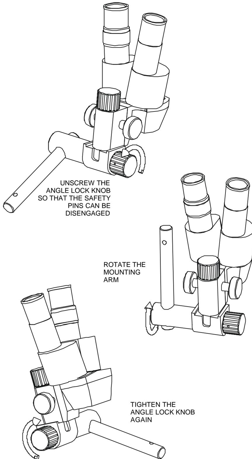
Figure 12b Changing the assistant microscope configuration
