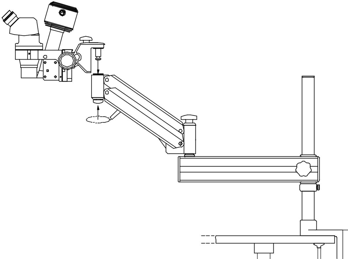
*Figure 5* Attaching the microscope assembly
