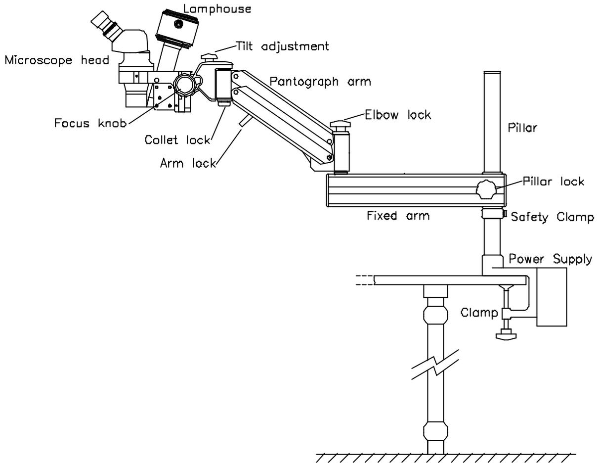
Figure 1 Scan Optics SO-161 Ophthalmic Microscope
