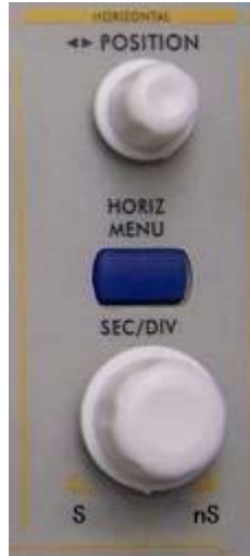
Fig. 4-10 Horizontal Control Zone
