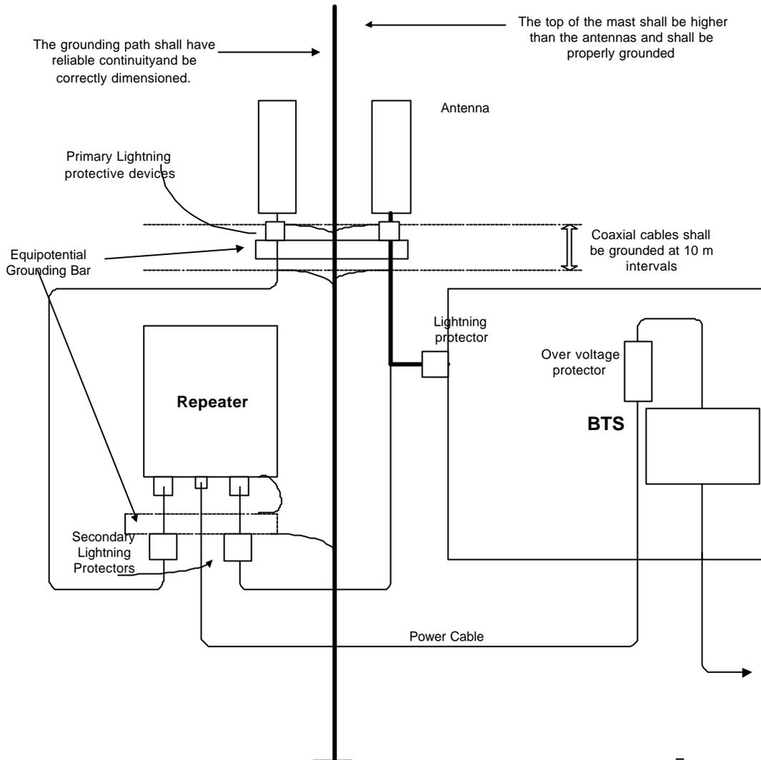
All coaxial cables and power cables need to be protected from the transients that lightning can cause.
