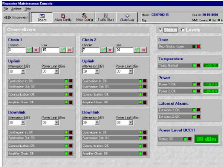
The channel and link fields have been filled in with carrier numbers 3, 15 ( chain 1) and 7, 20 (chain 2)
