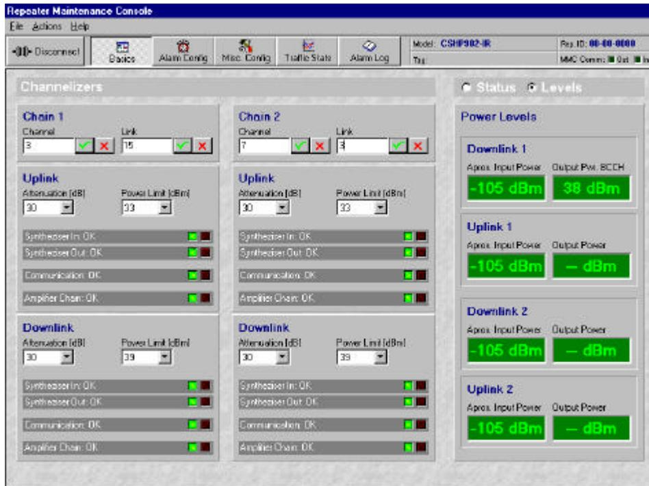
In the screen dump above the link carrier number in Chain 2 has been changed to carrier 3. The repeater will pick up the server antenna signal via the link antenna. The antenna isolation is the difference between 1 and 2. In this case  $38 - (-105) = 143\text{dB}$  (This is far more than the required 75dB which means that the antenna isolation is good)
