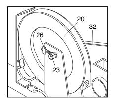
counterclockwise. Make sure that the Flywheel is straight and retighten the M10 Nuts (23). When the Drive Belt is properly adjusted, re-attach the side shields.
