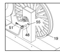
(30, shown removed for clarity). Slide the Reed Switch slightly toward or away from the Magnet. Make sure that the Magnet will not hit the Reed Switch. Retighten the Screw. Turn the Pulley (19) for a moment. Repeat until the console displays correct feedback. When the Reed Switch is correctly adjusted, re-attach the left side shield.
