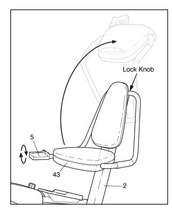
To switch from elliptical crosstrainer to recumbent bike, loosen the lock knob (not visible). Fold the Seat (43) down and turn the Console (5) so it is visible when you are sitting on the Seat.
