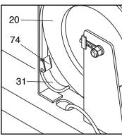
Buckle and turn the Flywheel (20) to make sure that there is not too much resistance. When the Resistance Strap is properly adjusted, re-attach the left side shield.
