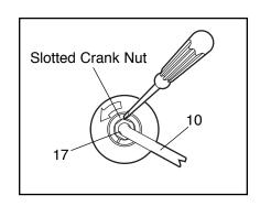
a hammer to turn the Slotted Crank Nut counterclockwise until the arms are no longer loose. Do not overtighten the Slotted Crank Nut. When the Slotted Crank Nut is properly tightened, retighten the Crank Nut and re-attach the left side shield.
