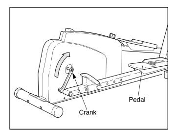
To dismount the REBEL, allow the pedals to slowly come to a stop. CAUTION: The REBEL does not have a freewheel; the pedals will continue to move until the flywheel stops. When the pedals are stationary, step off the highest pedal first. Then, step off the lowest pedal.
