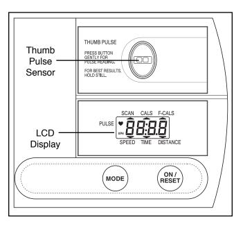
SPEED-This mode displays your pedalling speed, in miles per hour.
