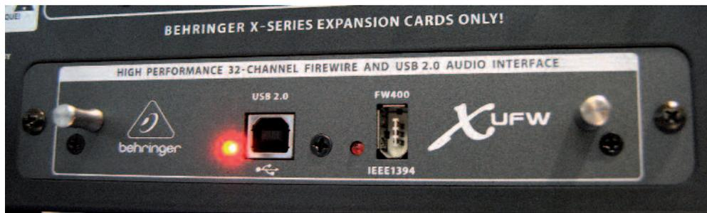
The XUF recording card is included and offers 32 channels in duplex mode (in & out), either to USB or FireWire
