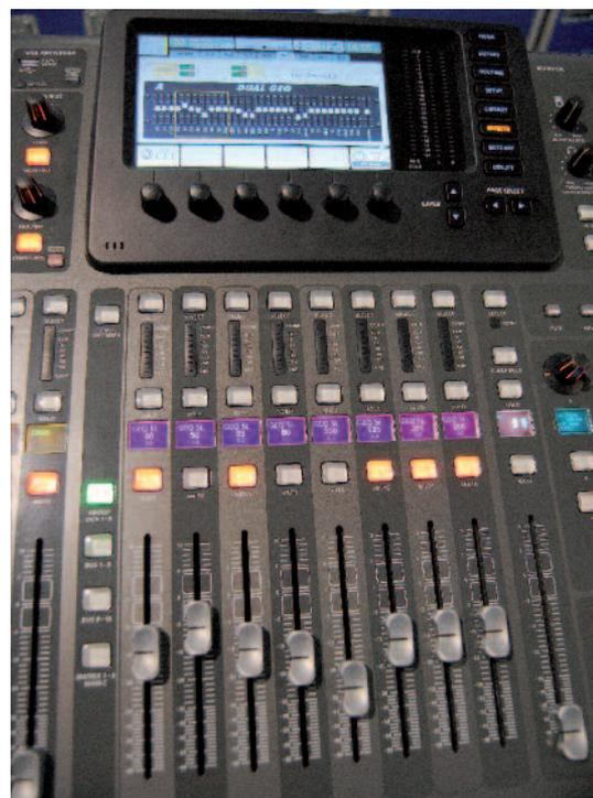
The fader of the DCA/bus section can also be used to drive the internal GEQs, the LCD displays thus show frequency, gain and channel to the selected GEQs
