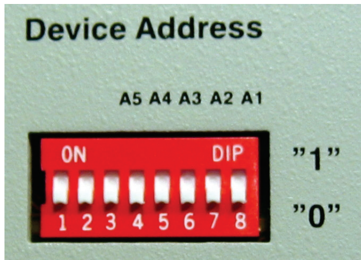
Fig. 2.5. Dipswitch settings binary "0"
