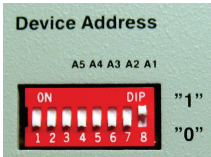
Fig. 2.6 Dipswitch settings binary "1"
