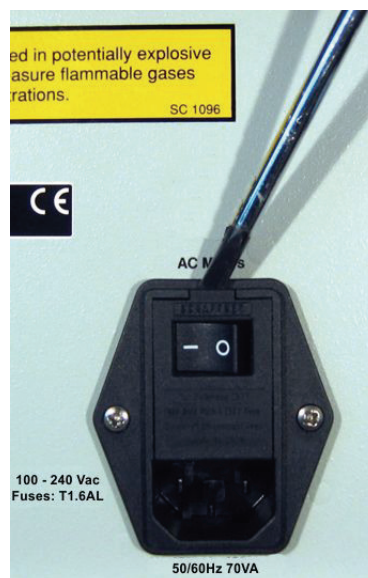
Fig.2.1. Accessing the 1309's fuses
