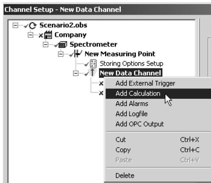
Figure 56: Pop-up menu on *New Data Channel* level
