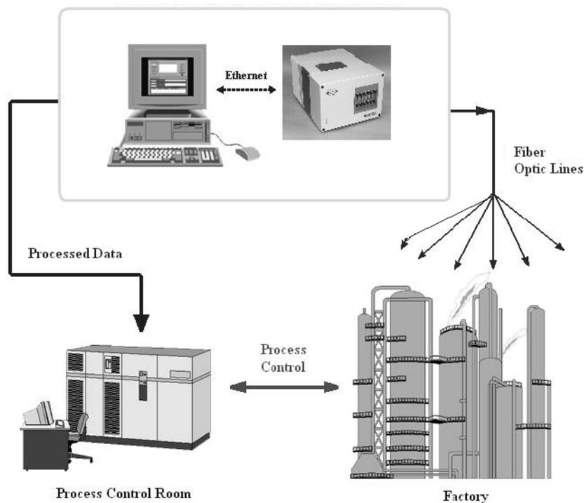
Figure 1: Process Control Setup
