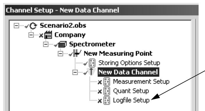
Figure 69: *Logfile Setup* sub-level in the browser
