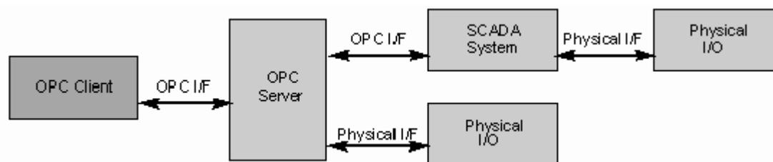
Figure 80: OPC client - OPC server architecture in an industrial information system
