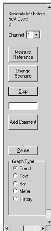
Figure 12: Process Control - control elements
