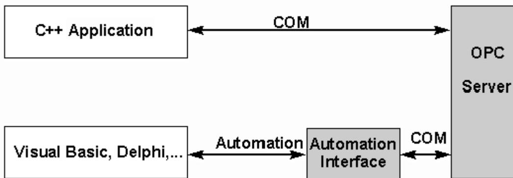
Figure 81: OPC scheme to use the automation interface wrapper connection link
