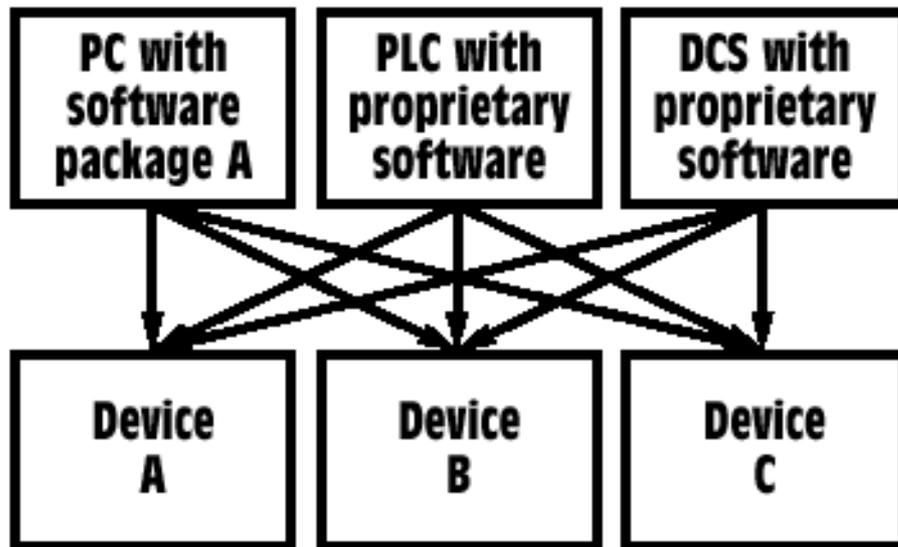
Figure 78: Scheme of an I/O driver problem
