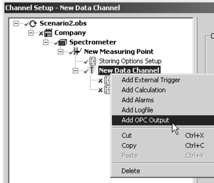
Figure 60: Pop-up menu on *New Data Channel* level
