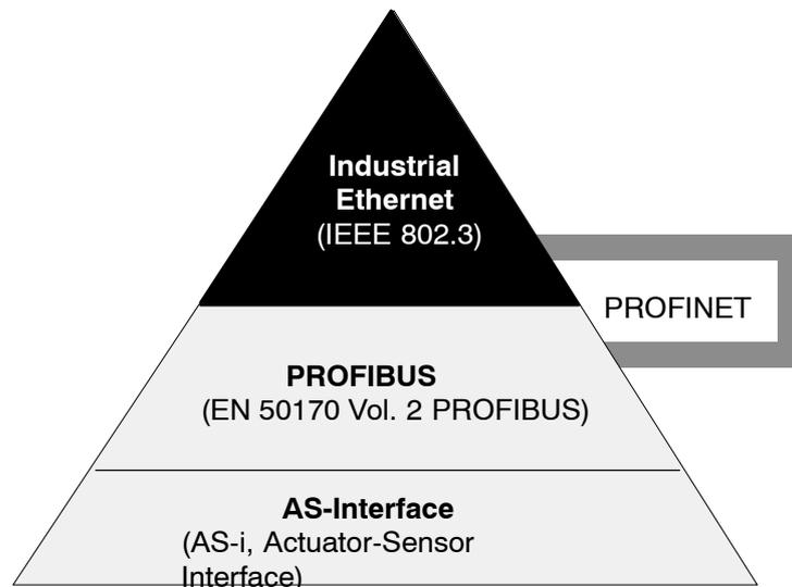
Figure 1-1 Industrial Ethernet in the SIMATIC NET concept
