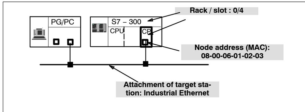
Figure 12-1 CP requiring diagnostics can be reached directly
