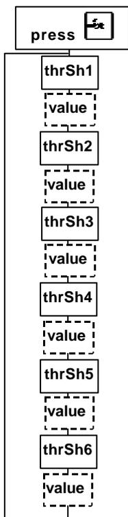
When viewing the menu, first the parameter name is displayed, then its value displayed when going to the following element.
