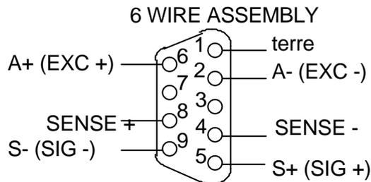
In the “4-wire” diagram, do not forget to use a strap to link the supply leads to the returns, as above. It is preferable to use the 6-wire set-up to neutralise weight drift caused by temperature variations that influence the voltage drop across supply leads from sensor or sensors.
