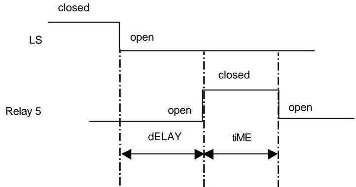
To adjust relay 5 time delays:
