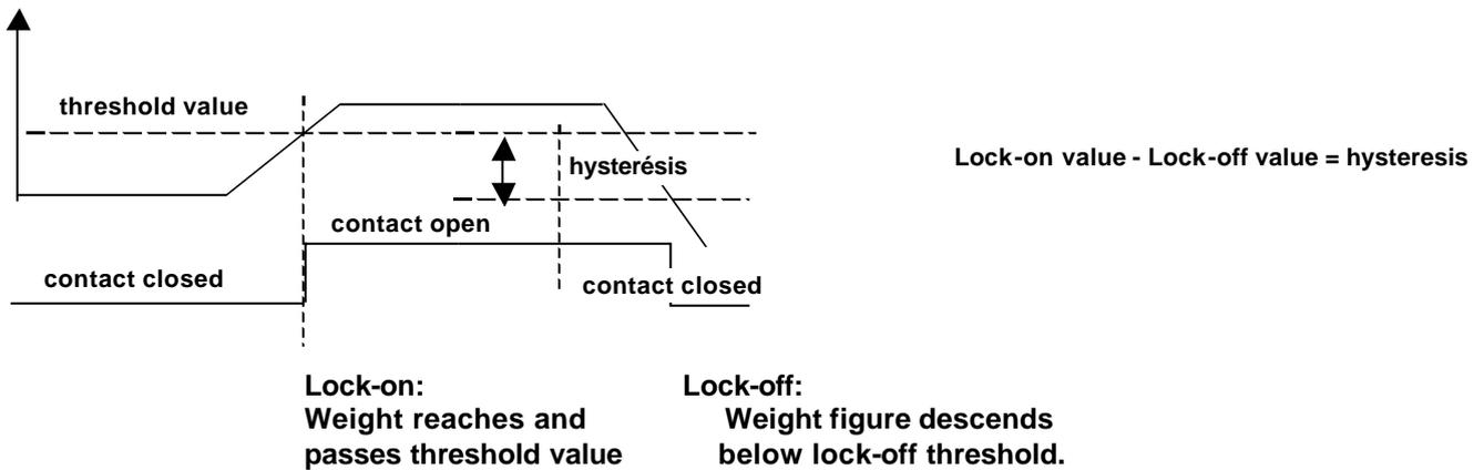
Threshold relay functioning can be associated with gross or net weight figures.
