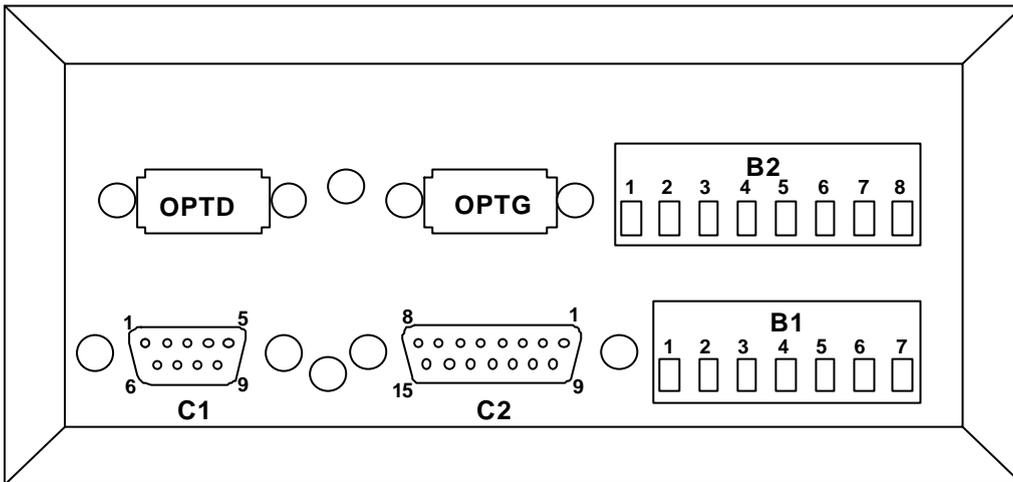
In its standard configuration the MS100 has one single card placed in the lower part. Terminal block B1 and main C1 and C2 connectors are on this card
