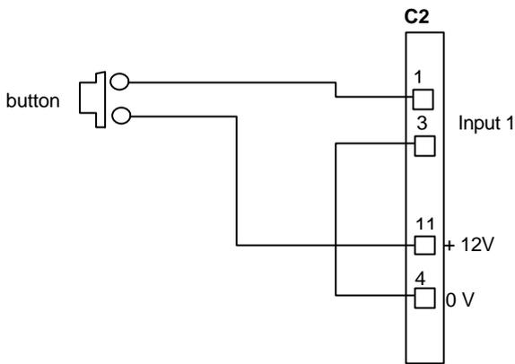
Relays 2 or 6 can be programmed by the installer to respond to a request from the remote control. The response diagram is as follows:
