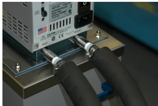
Hoses assembled to barbed fittings
