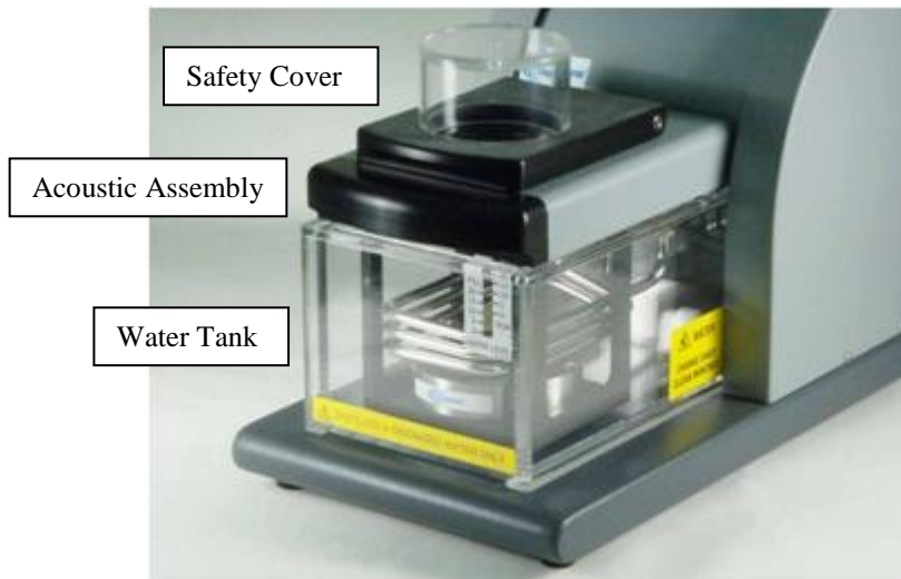
The S220 Acoustic Assembly and Water Tank
