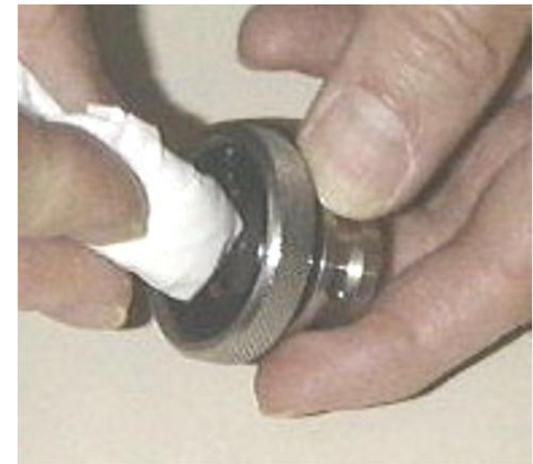
Cleaning end windows from furnace workhead
