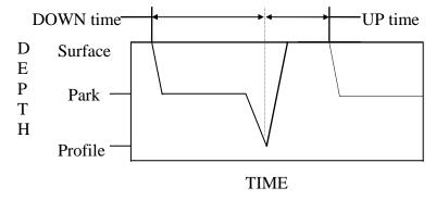
Parameter **PD** determines the frequency of deep profiles. Schematic examples:
