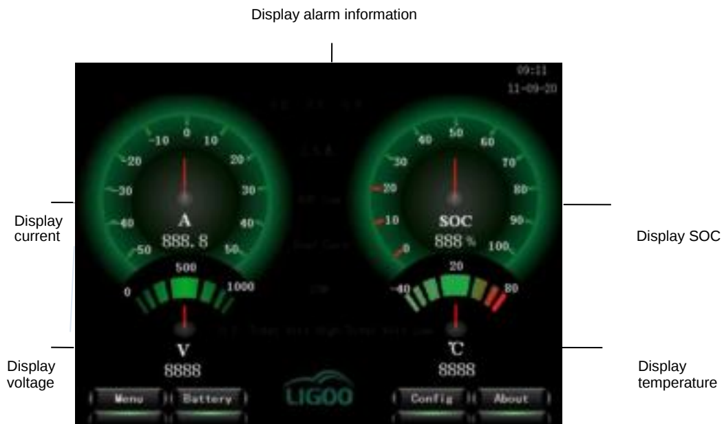
Figure 4-1 Main Interface of Terminal User
