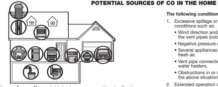
Fuel-burning appliances like: portable heater, gas or wood burning fireplace gas kitchen range or cooktop, gas clothes dryer. **Damaged or insufficient venting:** corroded or disconnected water heater vent pipe, leaking chimney pipe or flue, or cracked heat exchanger, blocked or clogged chimney opening.
