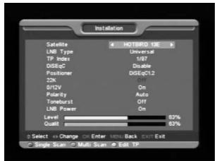
Positioner: In "Positioner" item, you can press [Volume Up/ Volume Down]key to switch "None / DiSEqC 1.2 / USALS" functions.
