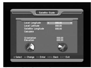
"Satellite Guide" is use for user to enter local longitude; local latitude and satellite longitude. By the evaluation from the receiver evaluate the antenna azimuth and antenna elevation; user can follow this guidance to adjust antenna.
