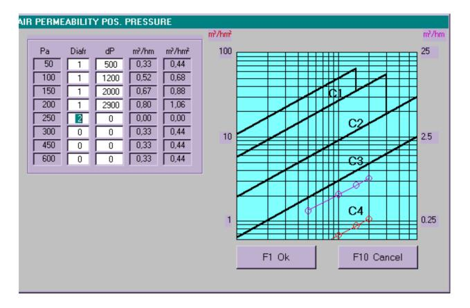
After the test is completed the machine waits to return to the main menu until confirmed with the "F1 Ok" button!
