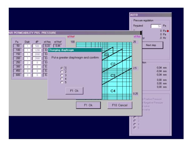
The way to choose a good diaphragm is to have a dP reading between 50 and 3000 Pa (the range of each diaphragm).
