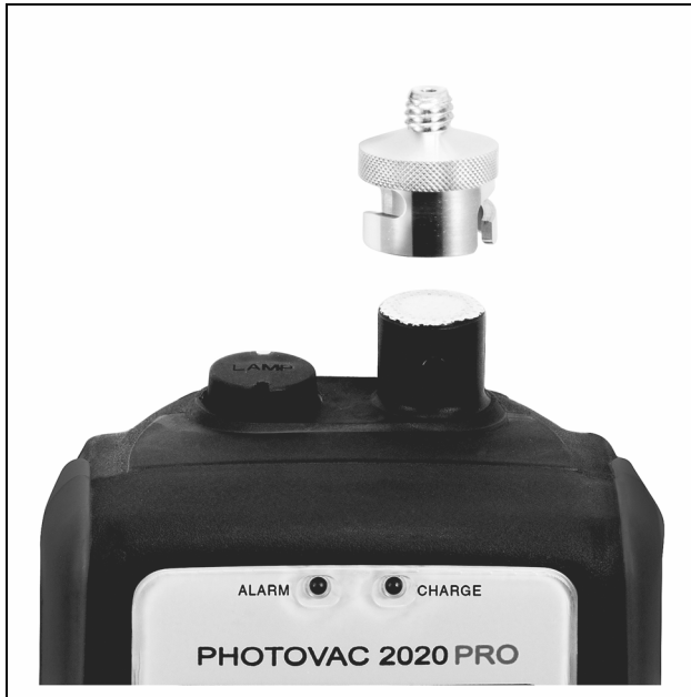
Figure 15. Replacing the Inlet Filter
