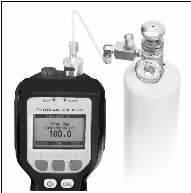
Figure 12. Calibration with Flow-Match
