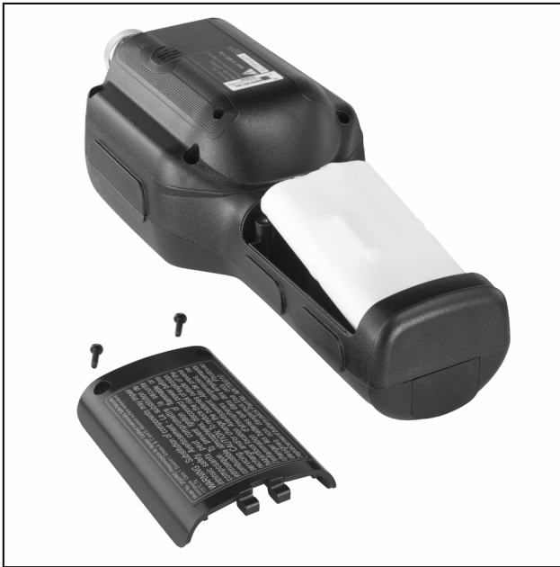
Figure 4. Battery Pack Removal and Replacement
