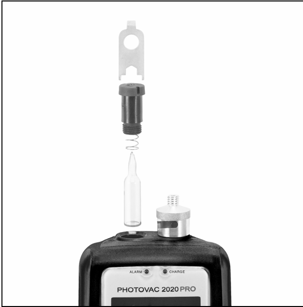
Figure 14. Removing the UV Lamp
