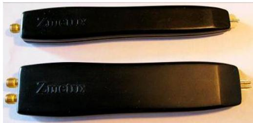
The ST600 is supplied with one single ended probe and one differential probe. The interior of the probe is a microstrip made of Rogers' material and the spring loaded probe pins have been selected for optimal performance. Standard pin separation is 0.100". Different pin spacing and/or configurations are available on special order
