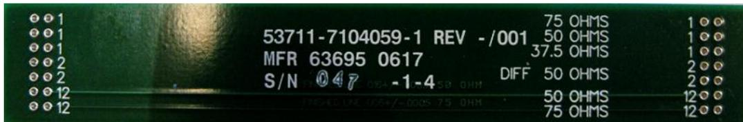
This coupon has six tracks to be measured, 5 single ended and one differential. The quickest and most efficient way to create a coupon test program is to make use of copy, paste and edit functions.
