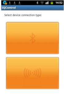
The button with a Bluetooth logo is used to control the device via wireless Bluetooth interface that needs to be turned on in your mobile phone.
