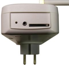
An integrated micro push button is located in the device, can be accessible through a round hole of 2 mm at the most outer side of your socket.
