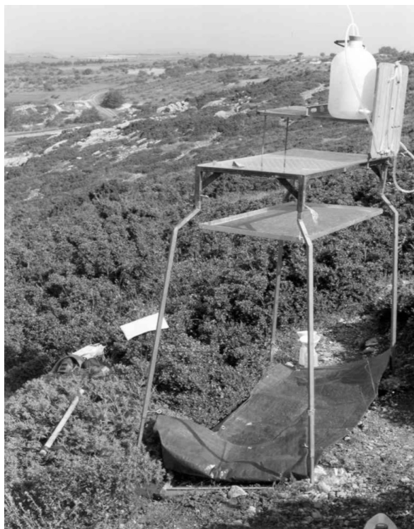
Fig 6. Portable rainfall simulator of Amsterdam type. Ready for use in the Petralona hills, in N Greece. Soil surface is covered with plastic to prevent wetting of surface while setting up the simulator. The rainfall dripping plate is 100 x 50 cm in size. Below the plate a randomiser is attached.
