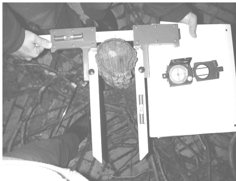
Fig. 11: Referencing of the root stump using spirit levels and compass
