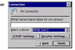
6. Enter the Host Name or IP address for a VPN connection, or a PPPoE Service Name for a PPPoE connection.
