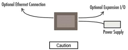
Electrical Shock Hazard: To avoid personal injury or damage to equipment, ensure that the DC supply is disconnected from power and that the leads are not energized before attaching them to the unit's power supply plug.
