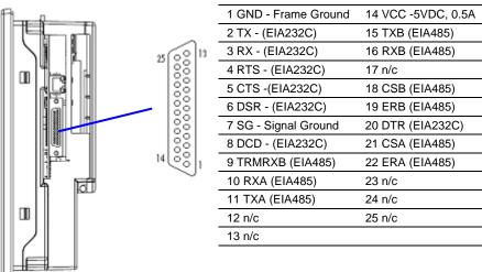
**Note:** Pin 14 is fused with a field-replaceable, 1.0A fast-blow fuse.
