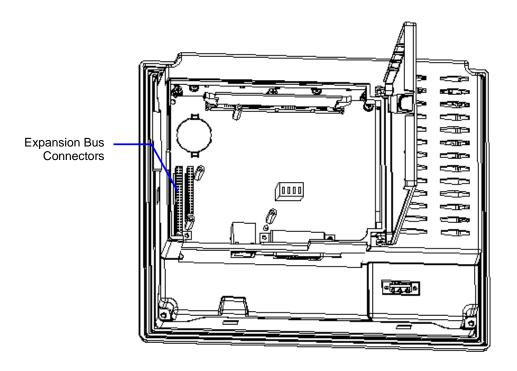
**Note:** To ensure compliance to CE Mark, the mounting screws must be used when installing an expansion card.
