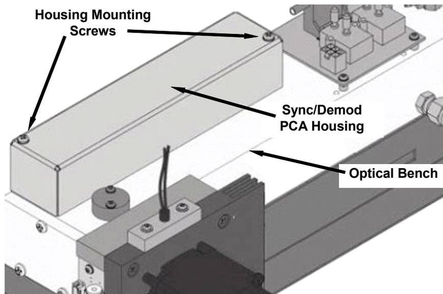
Figure 12-19: Location of Sync/Demod Housing Mounting Screws
