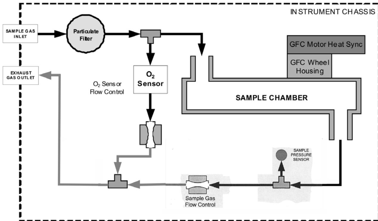
Figure 12-11: GFC7001T/GFC7001TM – Internal Pneumatics with O<sub>2</sub> Sensor Option 65A
