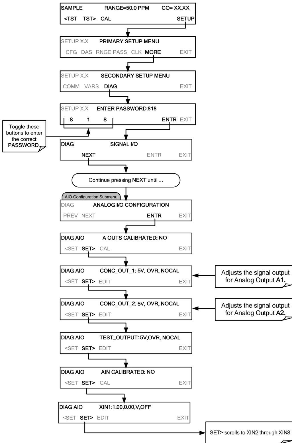
Figure 5-3: Accessing the Analog I/O Configuration Submenus
