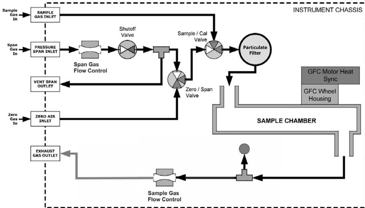
Figure 12-8: Internal Pneumatic Flow OPT 50B – Zero/Span/Shutoff Valves
