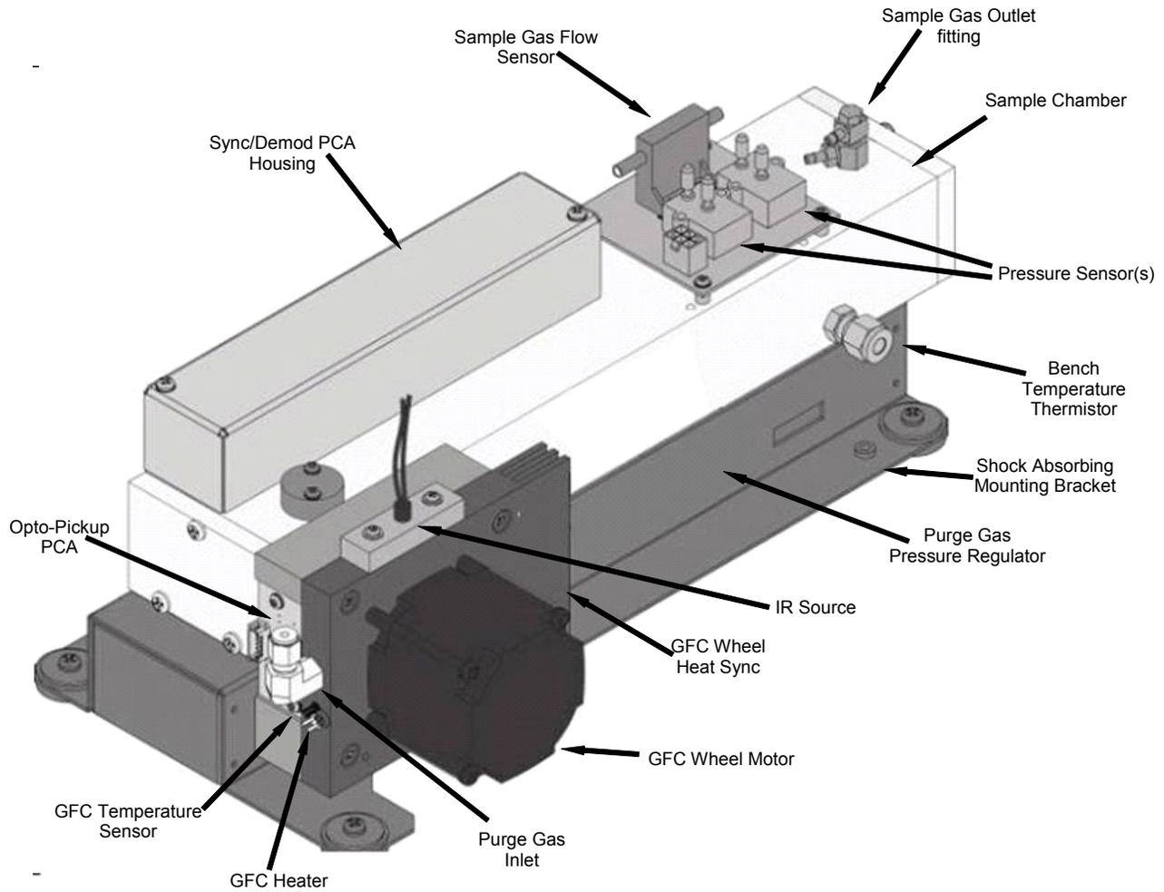
Figure 3-7: Optical Bench Layout (shorter bench, GFC7001TM, shown)
