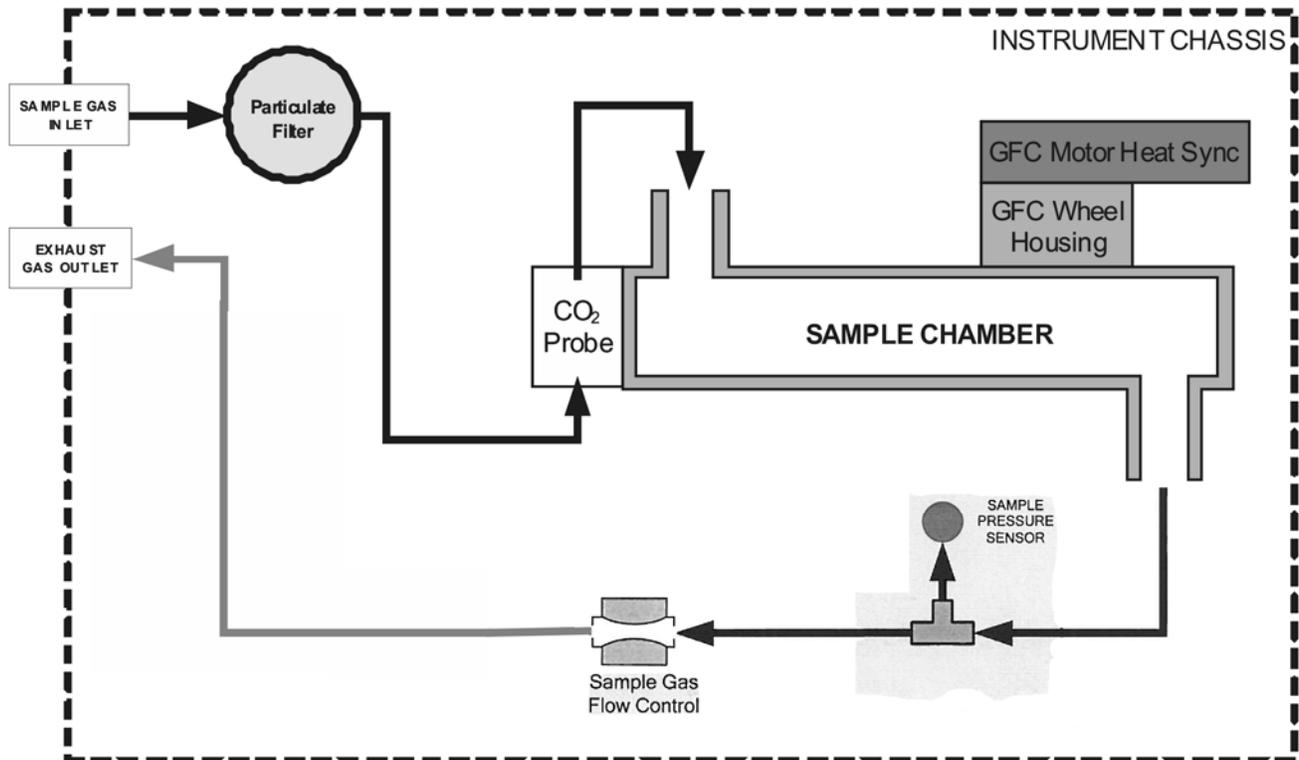
Figure 12-12: GFC7001T/GFC7001TM – Internal Pneumatics with CO<sub>2</sub> Sensor Option 67A
