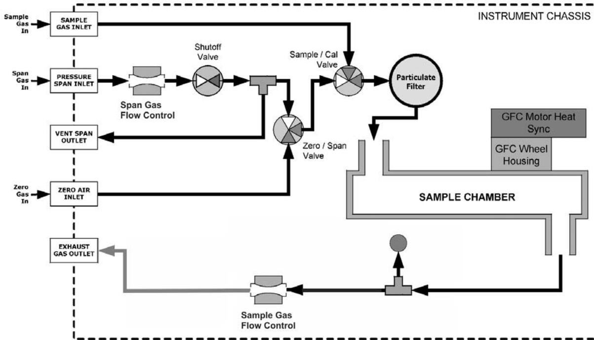
**Figure 3-23: Internal Pneumatic Flow – Zero/Span/Shutoff Valves (Opt 50B)**
