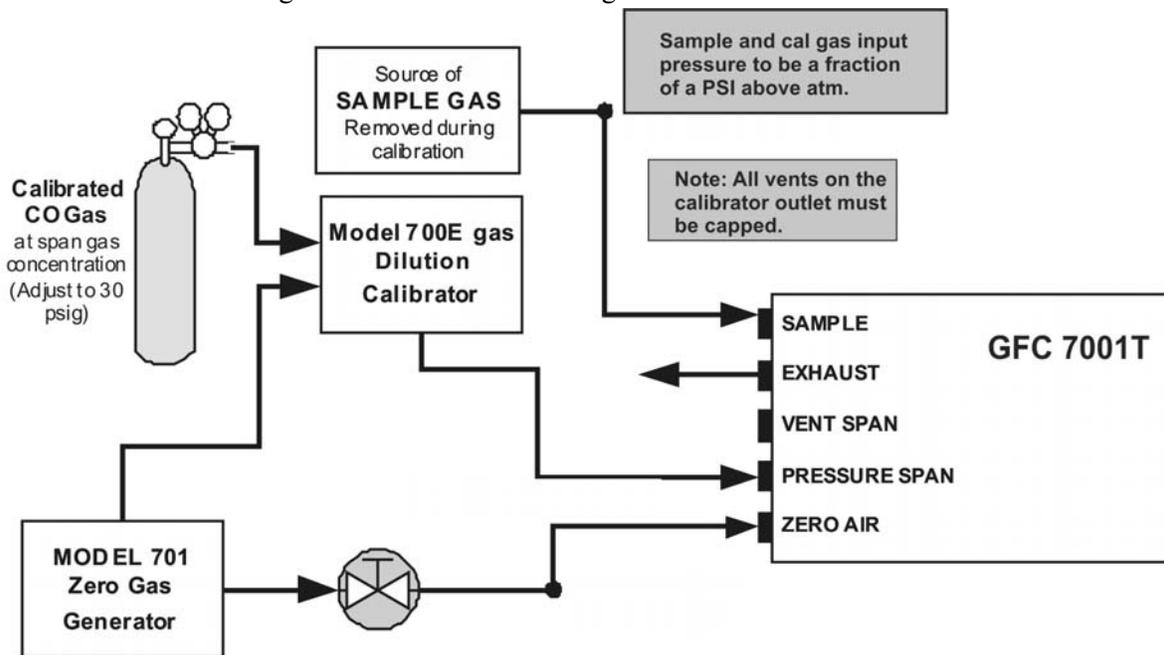
Figure 3-21: Pneumatic Connections – Option 50A: Zero/Span Calibration Valves
