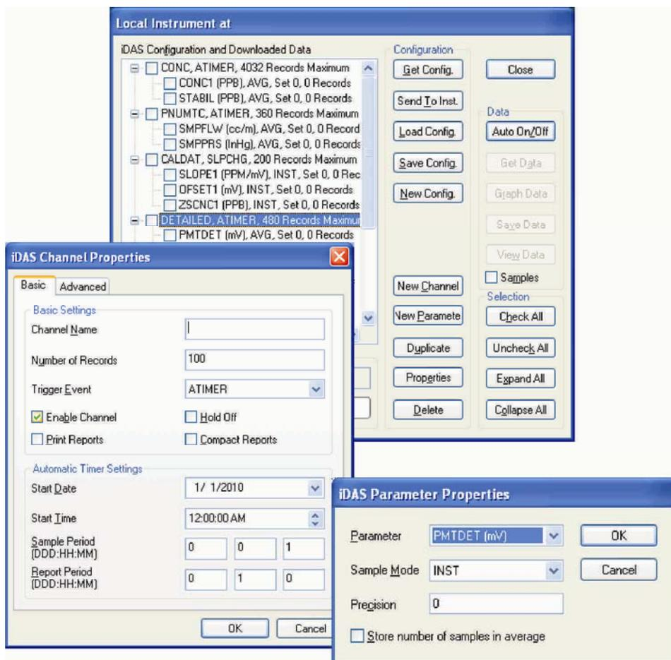
**Figure 7-3: APICOM User Interface for Configuring the DAS**
