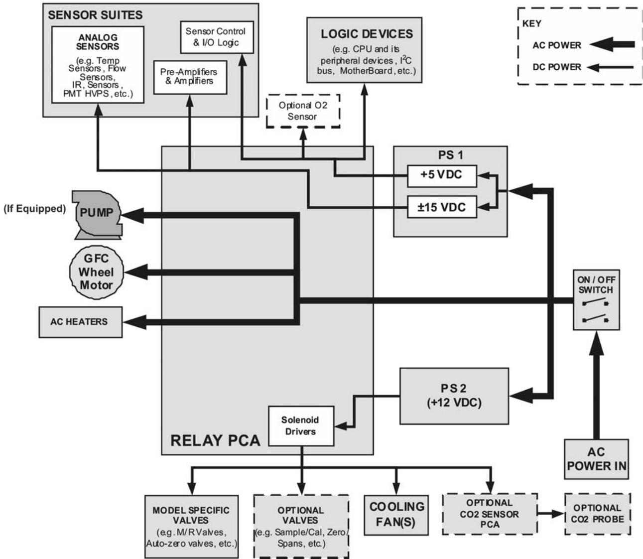
Figure 13-16: Power Distribution Block Diagram
