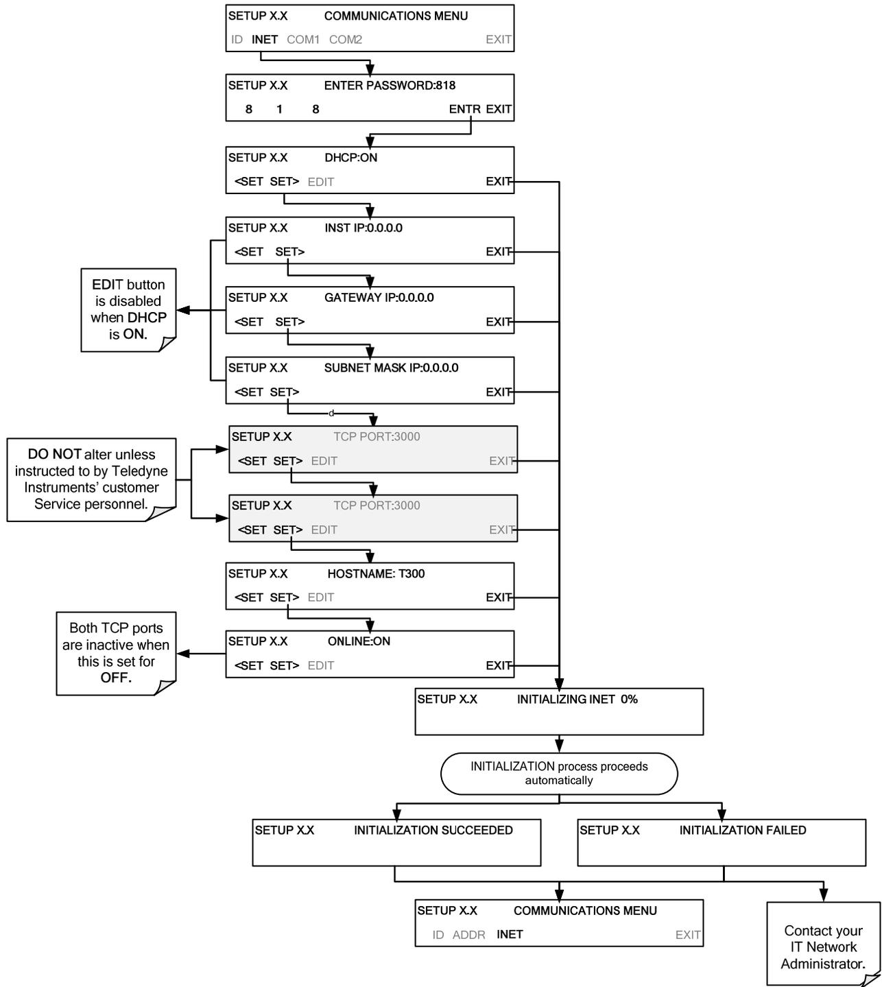
Figure 6-5 : COMM – LAN / Internet Automatic Configuration (DHCP)
