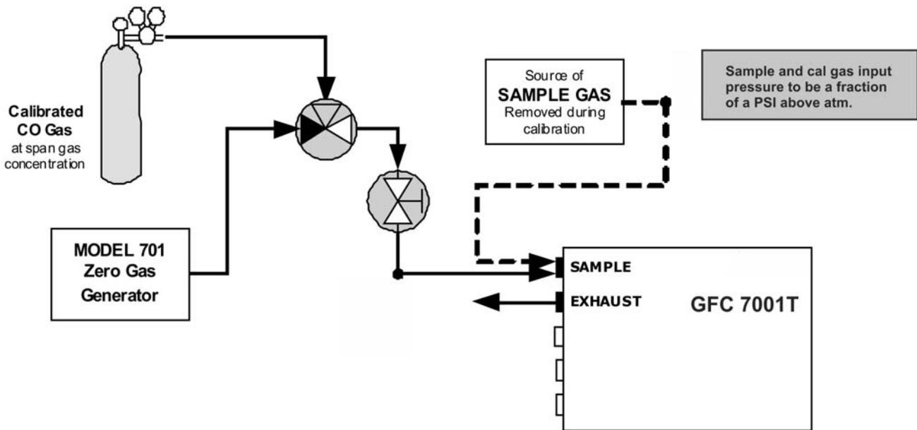
Figure 3-18: Pneumatic Connections–Basic Configuration–Using Bottled Span Gas
