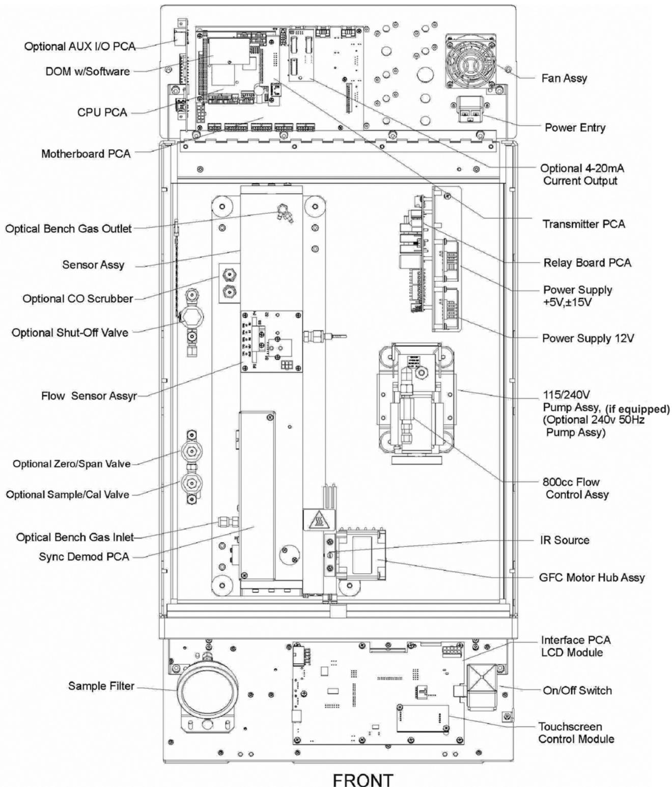
Figure 3-5: Internal Layout – GFC7001T
