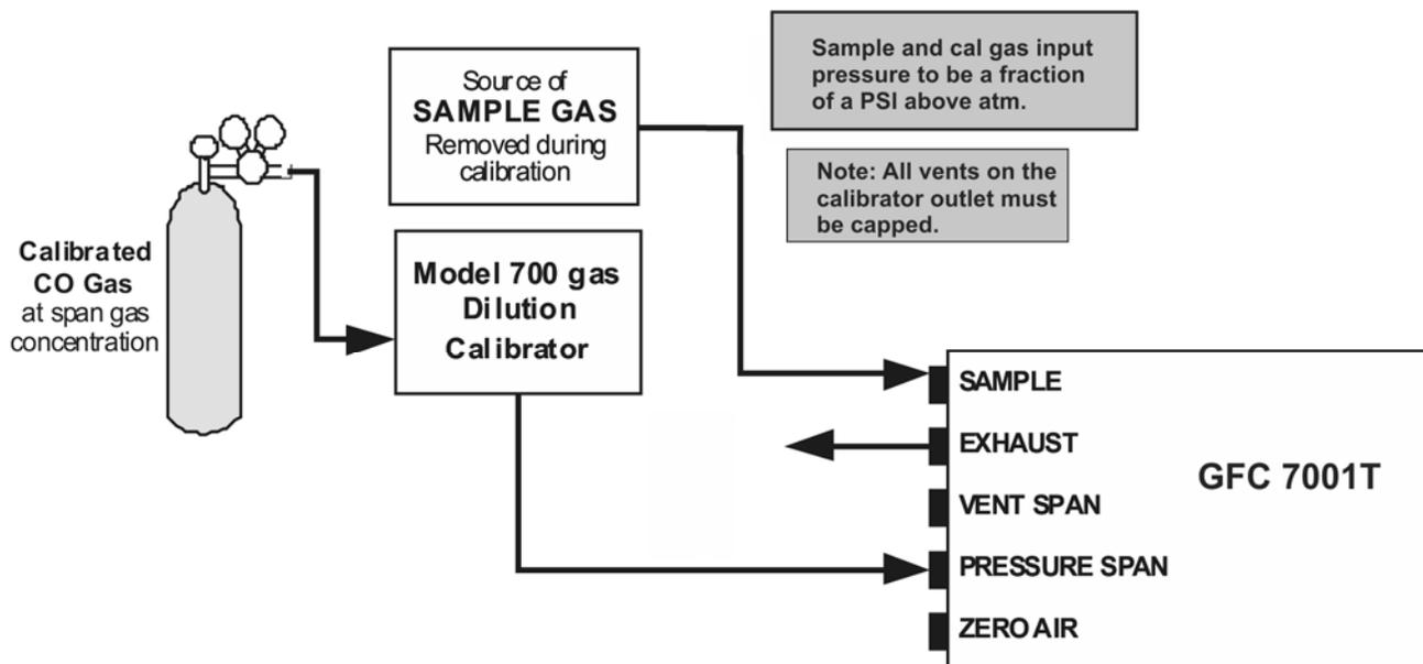
Figure 3-26: Pneumatic Connections – Option 50H: Zero/Span Calibration Valves
