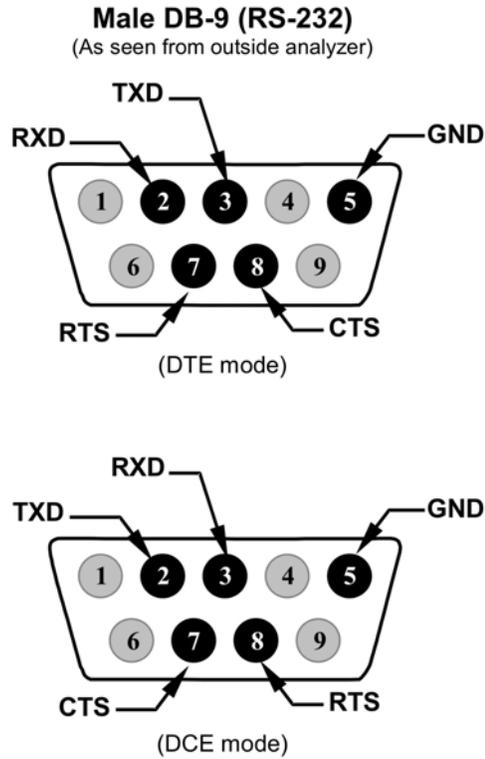
**Figure 3-14: Rear Panel Connector Pin-Outs for RS-232 Mode**
