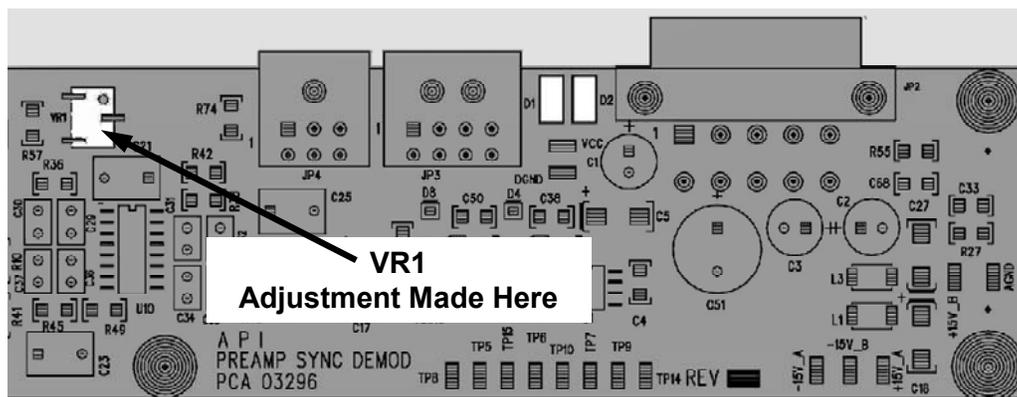
Figure 12-20: Location of Sync/Demod Gain Potentiometer
