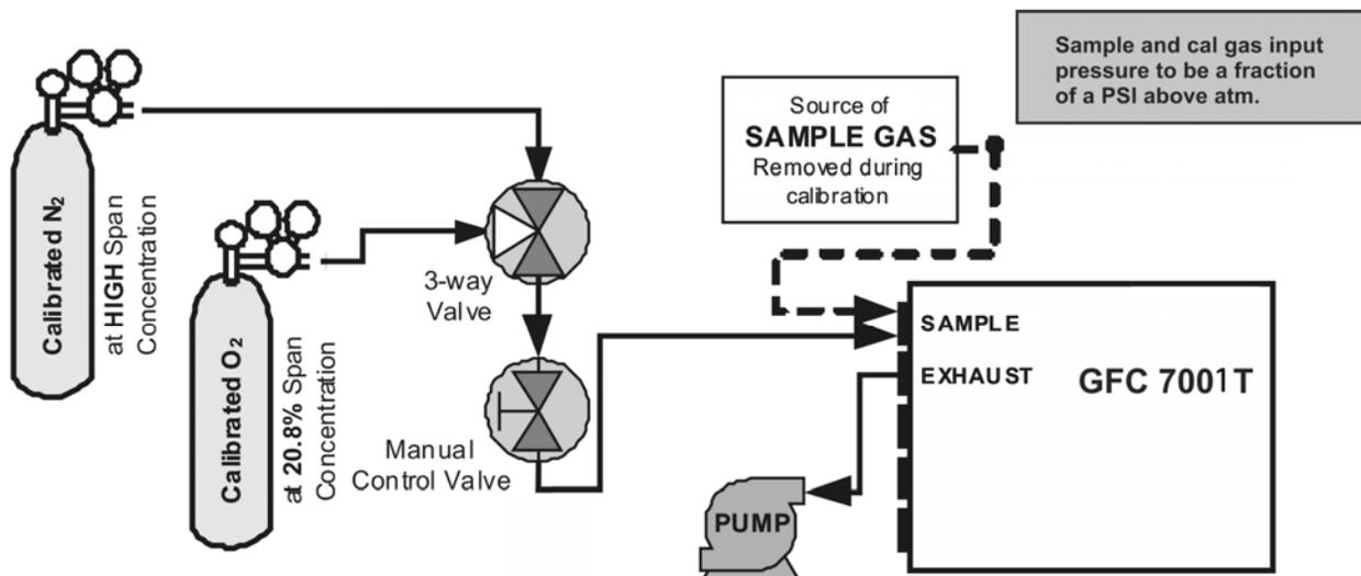
**Figure 9-7: O<sub>2</sub> Sensor Calibration Set Up**
