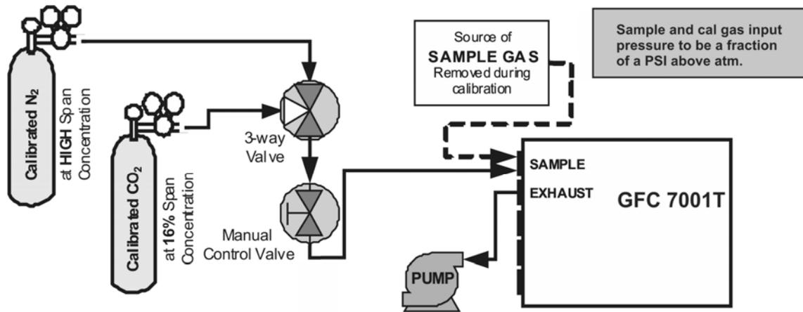
**Figure 9-8: CO<sub>2</sub> Sensor Calibration Set Up**
