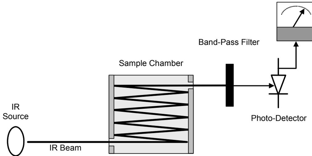
**Figure 13-1: Measurement Fundamentals**
