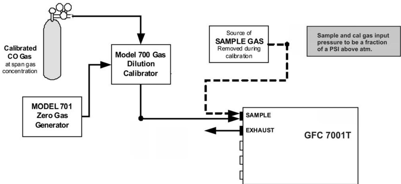
Figure 3-19: Pneumatic Connections–Basic Configuration–Using Gas Dilution Calibrator
