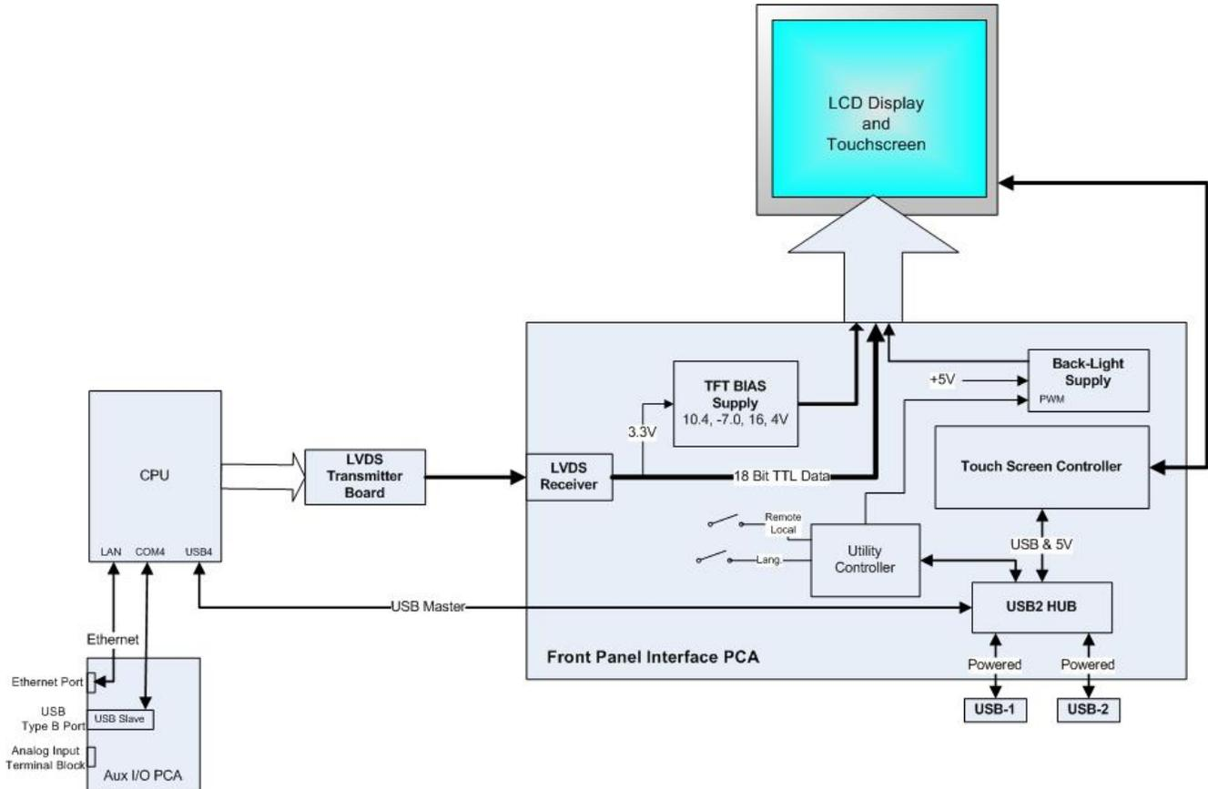
Figure 13-17: Front Panel and Display Interface Block Diagram
