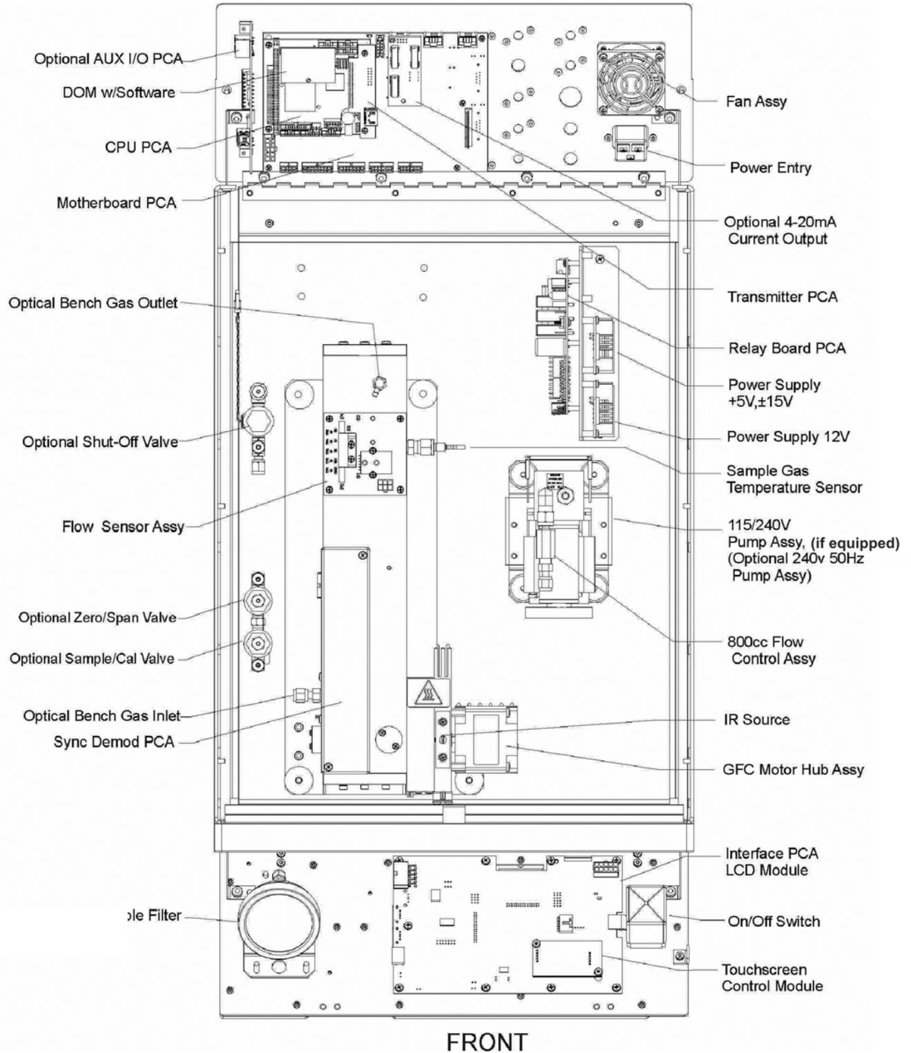
Figure 3-6: Internal Layout – GFC7001™
