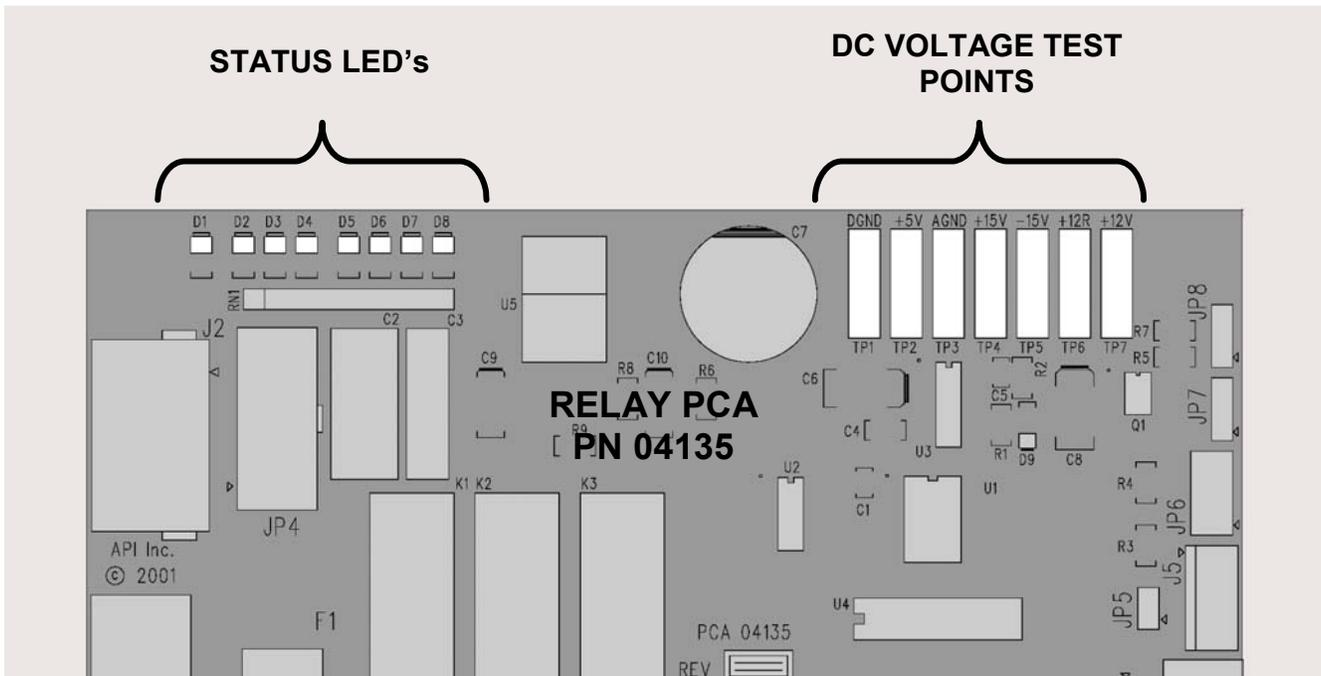
Figure 13-15: Location of relay board Status LEDs
