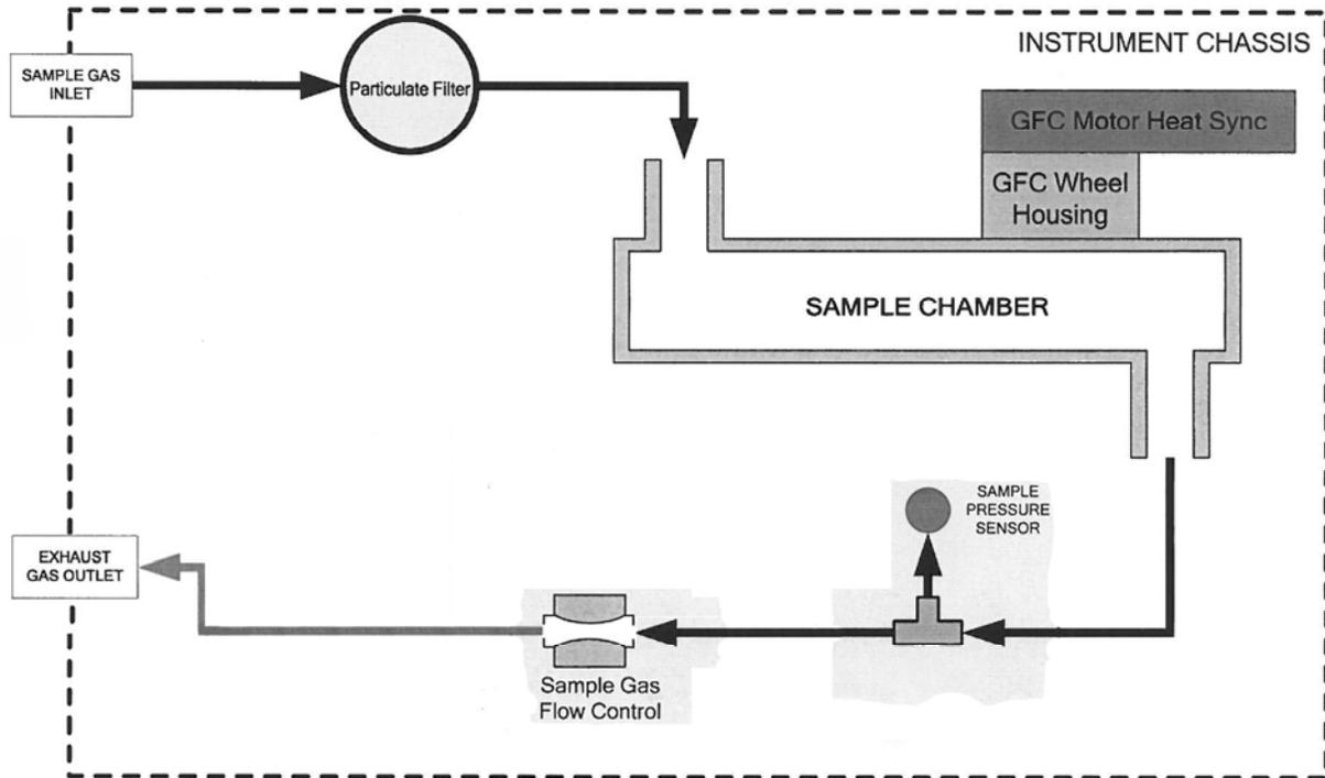
Figure 13-7: Internal Pneumatic Flow – Basic Configuration
