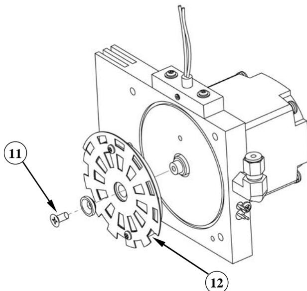
Figure 12-18: Removing the GFC Wheel
