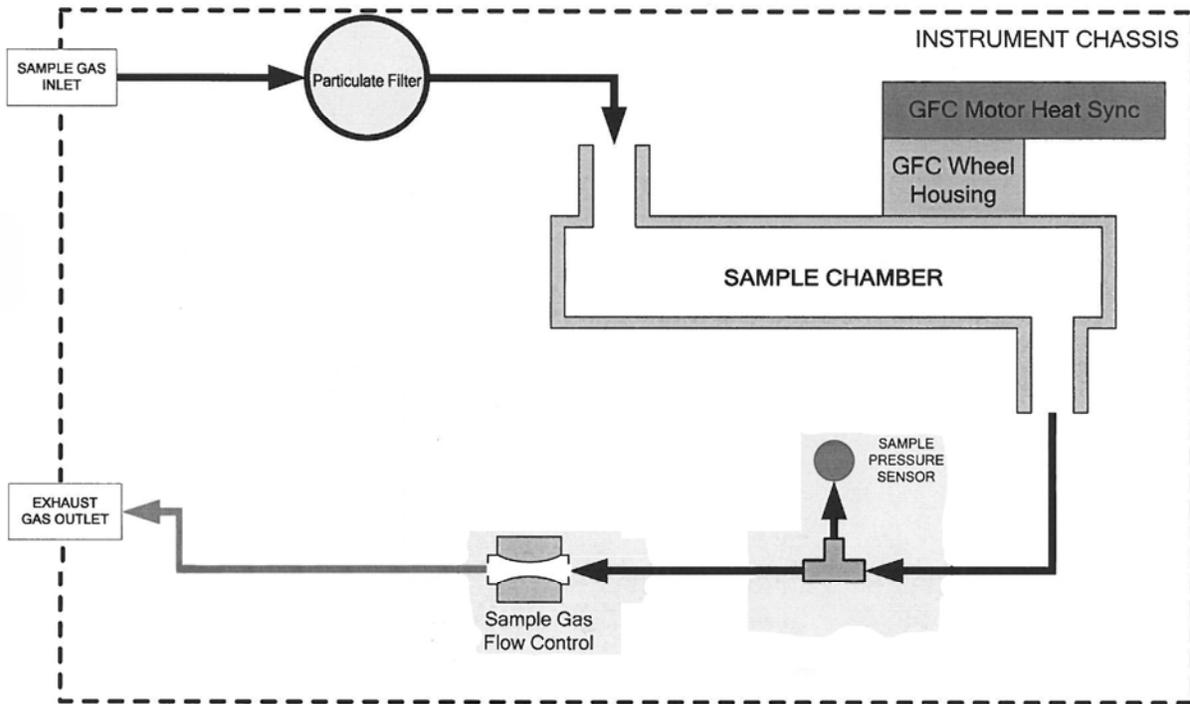
Figure 12-6: GFC7001T/GFC7001TM – Basic Internal Gas Flow
