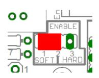
Hardware Enable will keep the driver enabled all the time.
