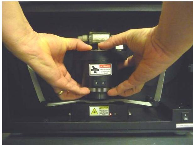
Figure 11. Manually Lifting the Chamber Optical Head
