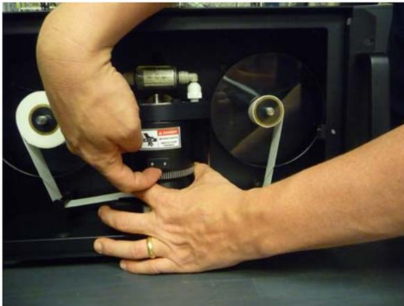
5. Use compressed air (AVOID spraying liquid) or to remove dust/debris from the optical head surfaces and platform.
