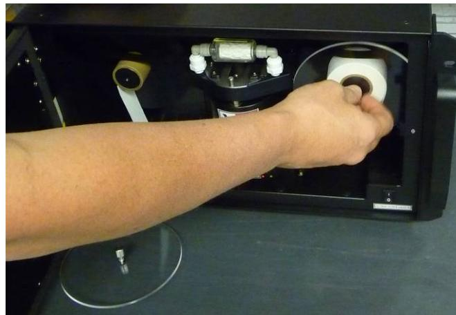
Slide tape from beneath the optical chamber and remove the used tape.
