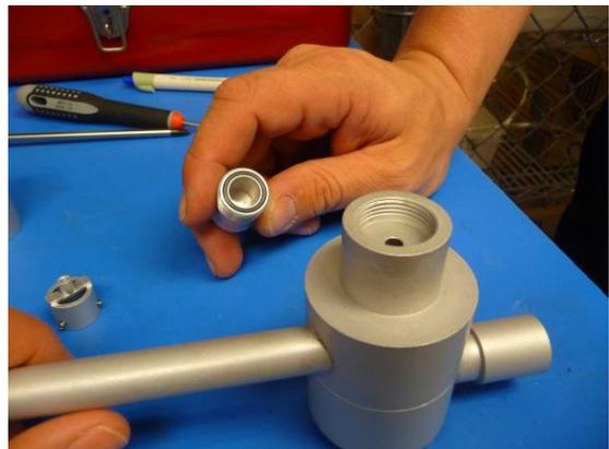
6. Illustration shows inlet cover, inlet body and dust cup removed.
