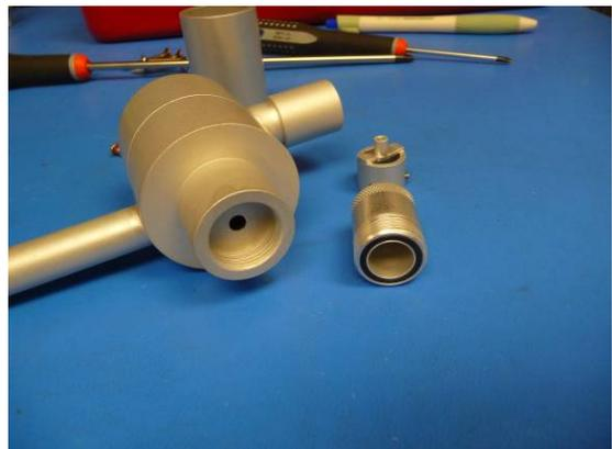
7. Remove allen cap screws from cyclone top.
