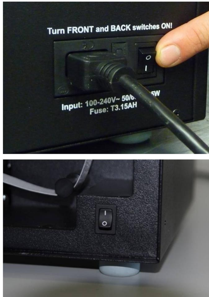
**Figure 8. Power on switches: rear panel (top photo) and front inside the door on the right (bottom photo).** Upon start-up, the instrument will proceed through an initialization period which can take up to 5 minutes (Figure 9). Various subunits are tested during this period and test results are
