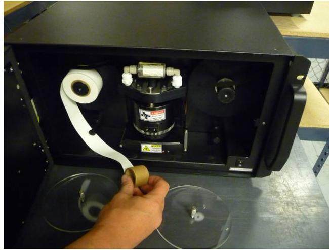
Slide the tape under the optical head,
