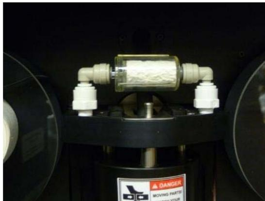
2. Hold down bottom fitting on one side while pulling up on cartridge fitting.
