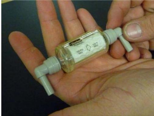
9. Place new cartridge on chamber optical head, ensuring that the arrow printed on the filter points to right.
