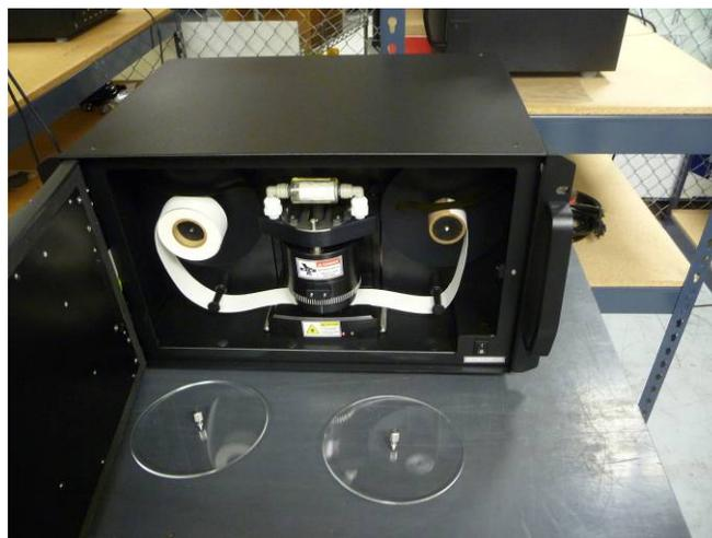
Ensure the tape is taut between the two sides.
