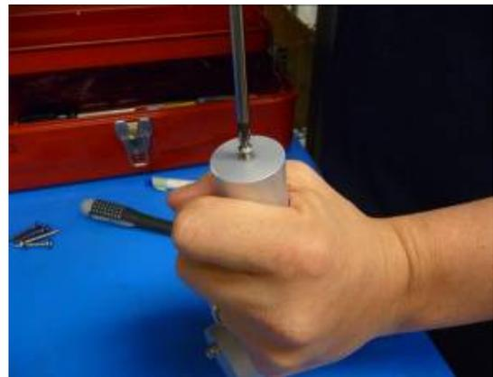
3. Loosen the three set screws that hold the inlet body in place.
