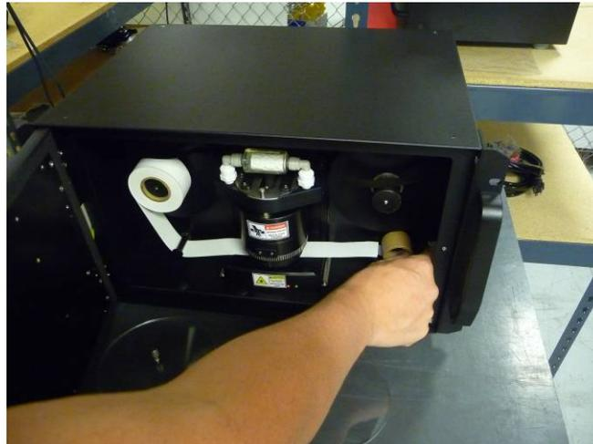
then run it under the right guide-arm and install the empty roll on the right. There may be some slack in the tape.
