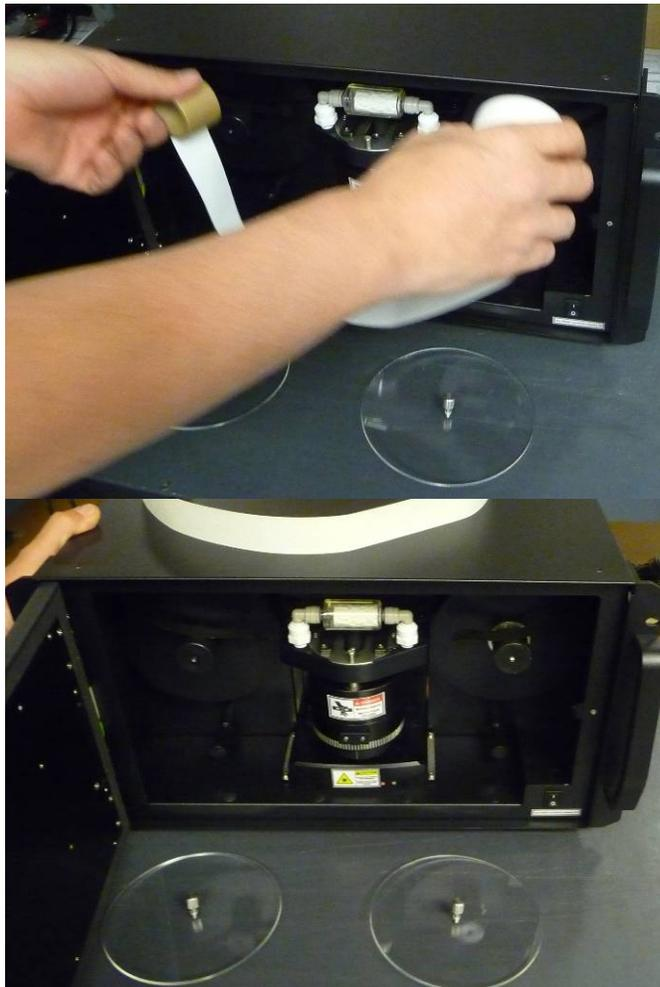
Using transparent tape, attach end of new tape to empty roll.
