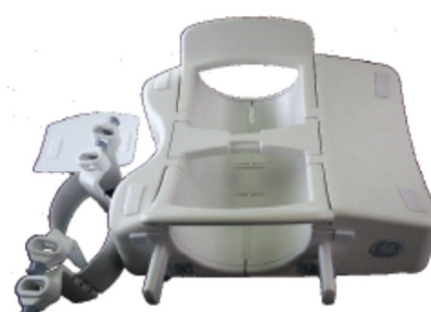
Dismount both retainers of the coil housing
