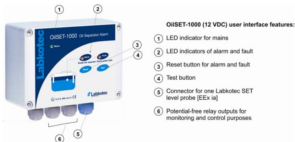
Figure 3. OilSET-1000 control unit – features
