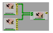
Next, connect the **AUTOSHIFT** to the top most **CLIP** Module. **CLIP** also needs the input vector layer, which you must connect to the Vector port.
