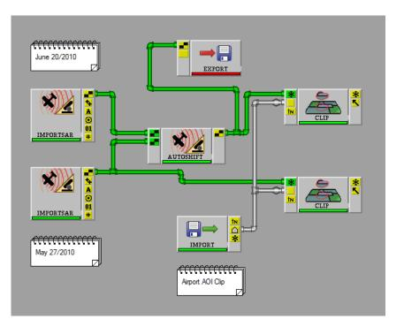
Note: For viewing purposes, you should connect the June 20<sup>th</sup> **AUTOSHIFT** results to the export module, which will allow you to see the original image, properly positioned and aligned with the other SAR image.
