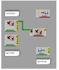
Repeat the step, this time connecting the **Reference Complex SAR Image** port on the Autoshift module to the May 27<sup>th</sup>, 2010 image.
