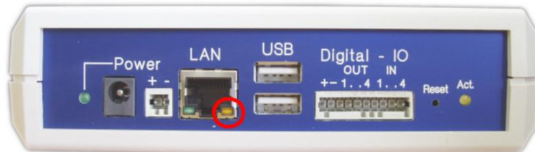
The physical interconnection is OK if the yellow link LED turns on when LAN cable is plugged in. The yellow light stays on until the connection breaks down. On some hardware models the link LED flickers synchronously to the green activity LED if there is traffic on the network line.
