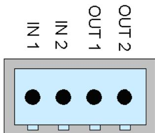
**Figure 2.8. Pin layout, digital IO plug (DIN rail model)**
