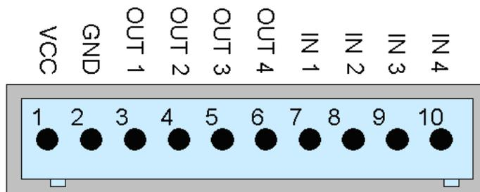
**Figure 2.7. Pin layout, digital IO plug (desktop model)**
