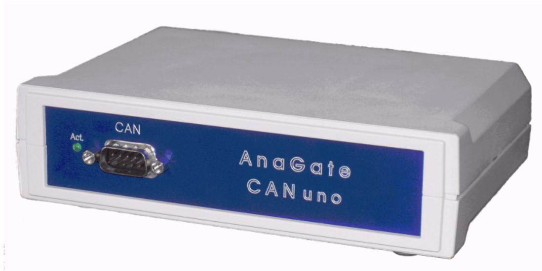
**Figure 1.1. Front view, AnaGate CAN uno**
