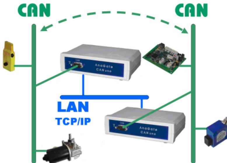
**Figure 3.2. AnaGate CAN Gateway in bridge mode**
