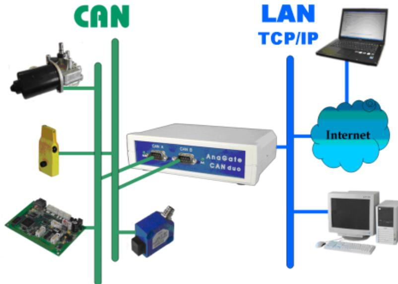
**Figure 3.1. AnaGate CAN Gateway in gateway mode**
