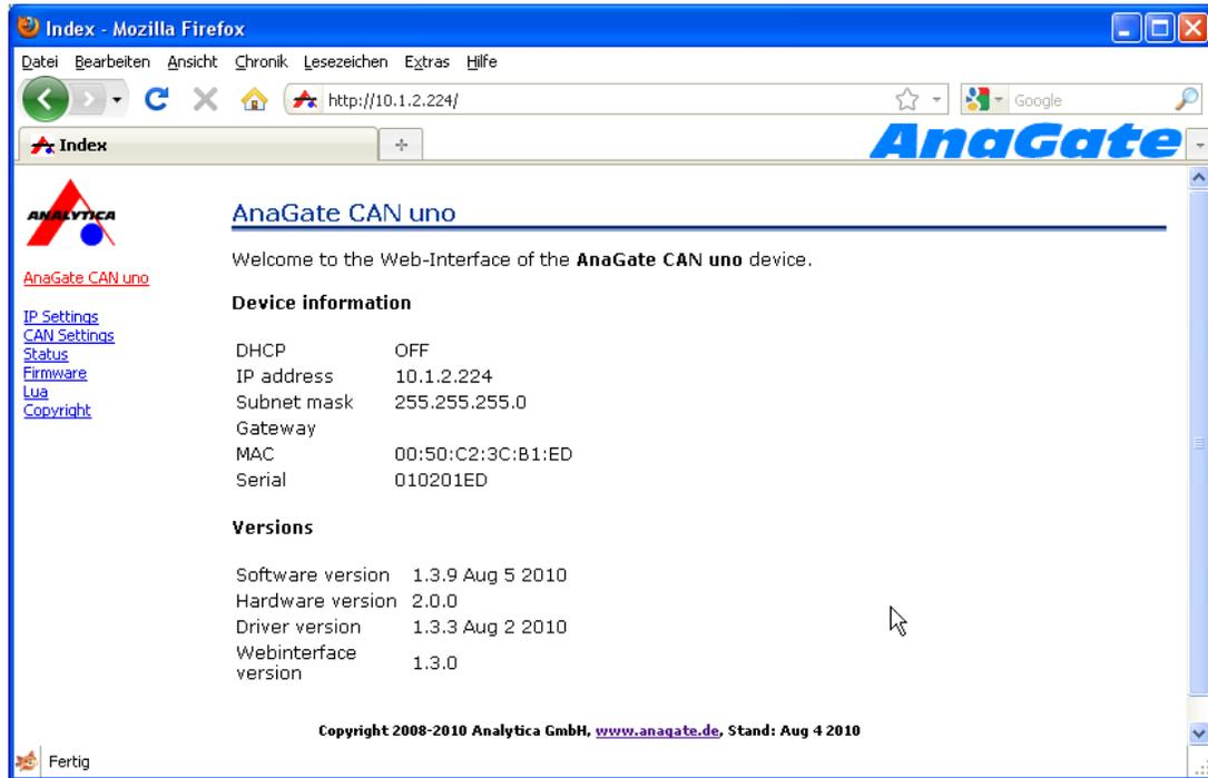
**Figure 2.10. HTTP interface, AnaGate CAN uno**
