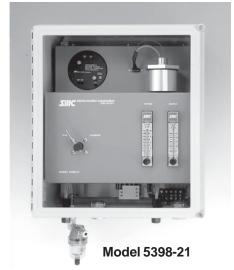
The Sample Draw Panels are intended for installation in an area, which is accessible, by the user for periodic routine inspection and calibration. The panel requires 120 VAC input and provides local visual as well as remote indication of pump and flow status.
