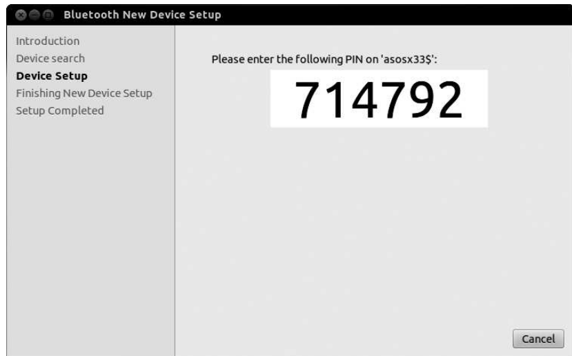
Figure 7-17: The Bluetooth wizard provides you with a PIN to input into the device you're pairing to.
