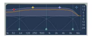
The Trans-X Wide shows a gain adjustment meter where the range is indicated by purple shading and a yellow line represents the gain adjustment within the range. The Trans-X Multi shows a similar display with a dynamic gain line over the full band spectrum so that you can see how much gain is adjusted per each band.
