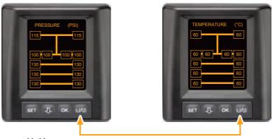
• Press the () button to change between the temperature display and the pressure display.
