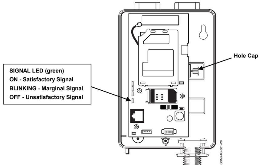
3. Verify the SIGNAL LED (green) remains steady for a few minutes, then mark that mounting position. Turn power off.
