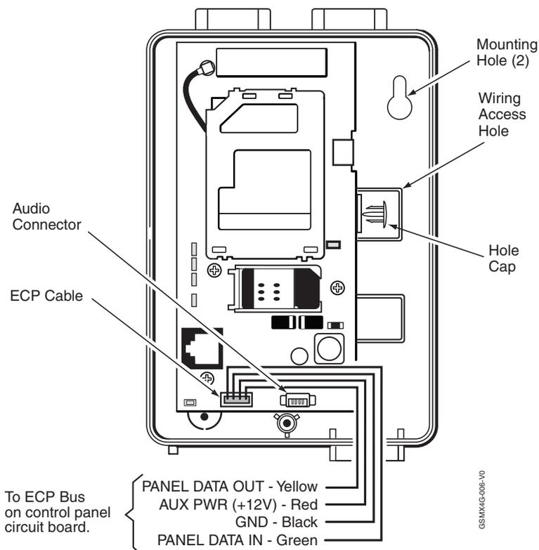
4. Connect the ECP cable to the communicator circuit board. When mounting the communicator off the cabinet, the length of the supplied ECP cable will have to be spliced to a four-wire extender cable. **Ensure the splices are located within the communicator's enclosure.**
