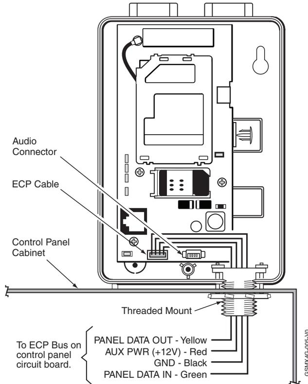
4. Connect the ECP cable to the communicator circuit board and thread the wires through the threaded mounting adapter.
