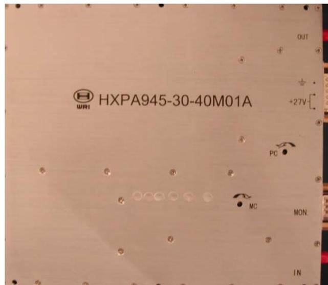
930MHz▯ 960MHz ALC Auto Level Control 40W Output Power Amplifier
