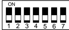
Figure 4. ST1, ST2 and ST3 DIP Switches with all switches in the OFF position.
