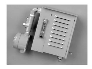
The Sierra Monitor Model 4400 provides the user with a low-cost, easy-to-use solution to effective monitoring of natural gas streams. This system accurately measures H<sub>2</sub>S concentration in the 0-100 ppm range. Fast response of 90% of step change within 30 seconds enables the user to respond quickly to changes in natural gas supply conditions to prevent product contamination.
