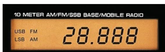
Liquid Crystal Display Panel: The liquid crystal panel provides the user with a visual information on the operation and status of the AE 497 W.
