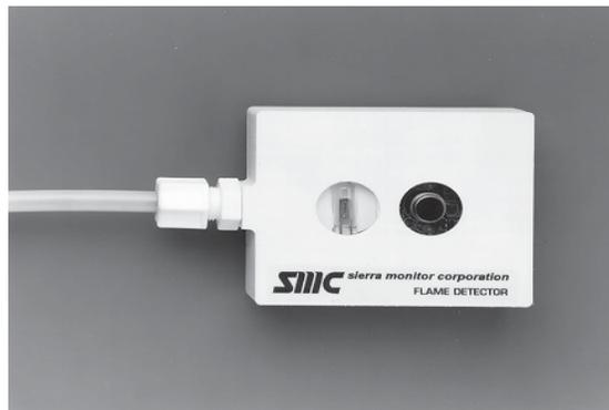
rejecting common false alarms. Continuous self diagnostics perform tests of the detector operation. Each flame detector is tested to respond to a 4-inch diameter isopropyl alcohol (IPA) fire at 10 feet with a 120° field of view.
