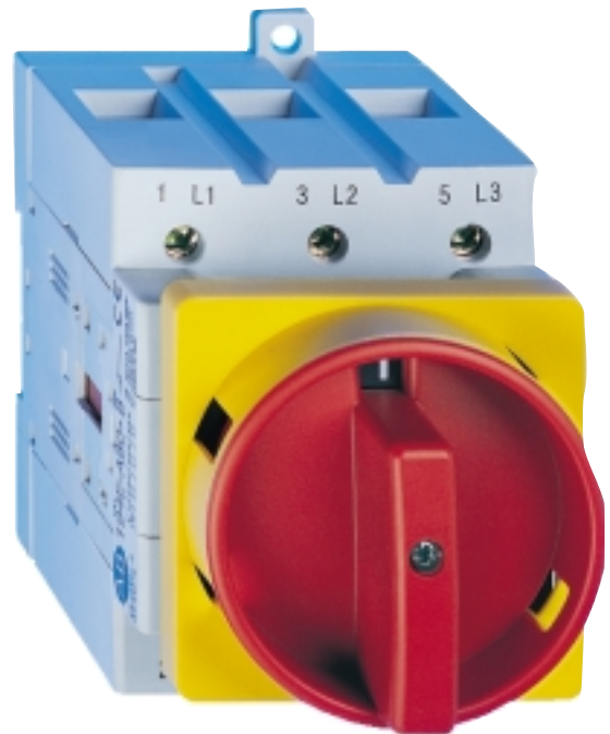
Control and load switch, which could be applied as a hand-operated disconnect or as an Emergency Stop when using the red actuator (as shown).
