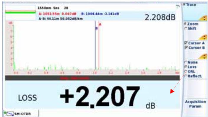
Fig. 12 Example of loss measurement between A & B cursors
