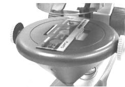
3. Next, choose the magnification strength you desire. In general, it is recommended to begin with lower magnification for easier focusing. To change the magnification setting, turn the magnification revolving turret until you hear a click.
