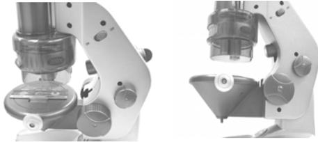
5. Look through the eyepiece and slowly adjust the focusing knob until the object on the slide becomes clear. To view different part of the slide, adjust the clip adjusters until the desired object appears through the eyepiece.
